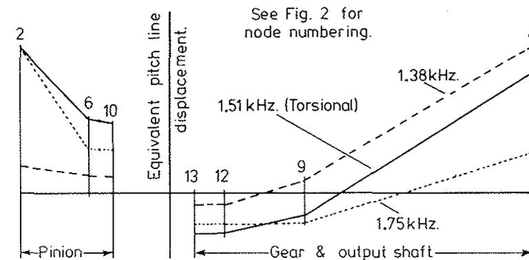
FIGURE 8 1.51kHz. TORSIONAL MODE WITH COMPARABLE OVERALL SYSTEM MODES
