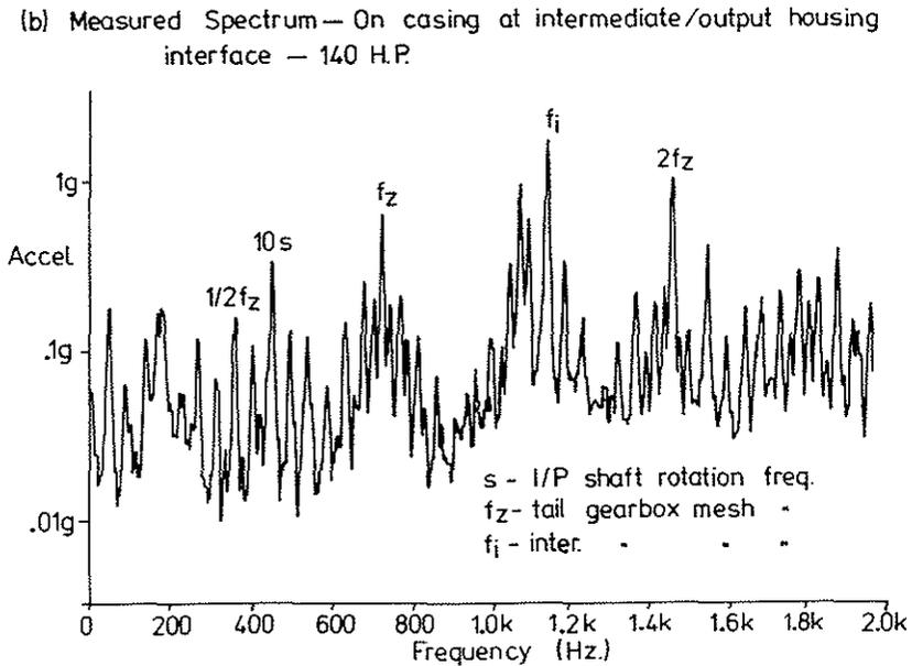
FIGURE 12 PREDICTED & MEASURED SPECTRA - 2730 R.P.M.
