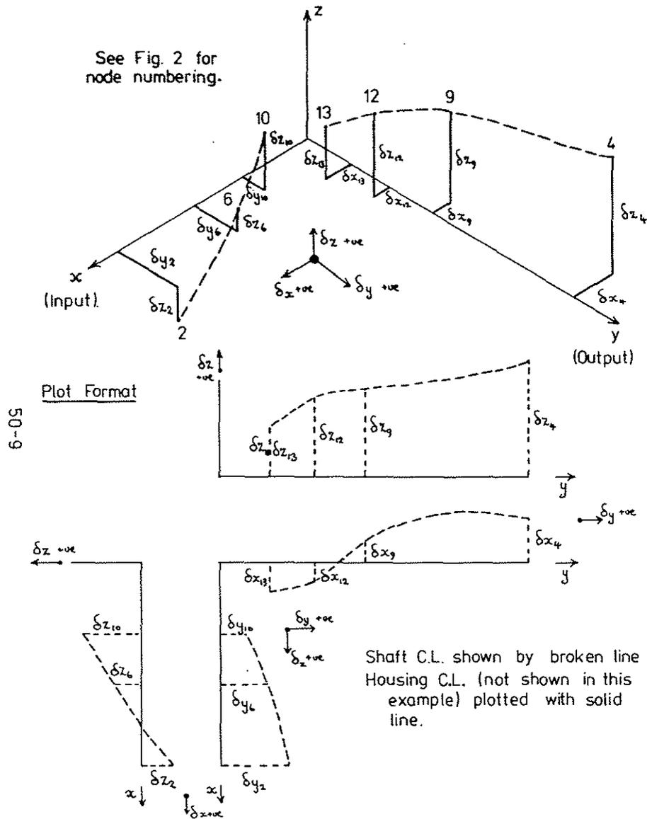
FIGURE 3 EXPLANATION OF PLOT AXES AND CONVENTIONS USED IN DEFLECTION & MODE PLOTS - FIGS. 4-7.
