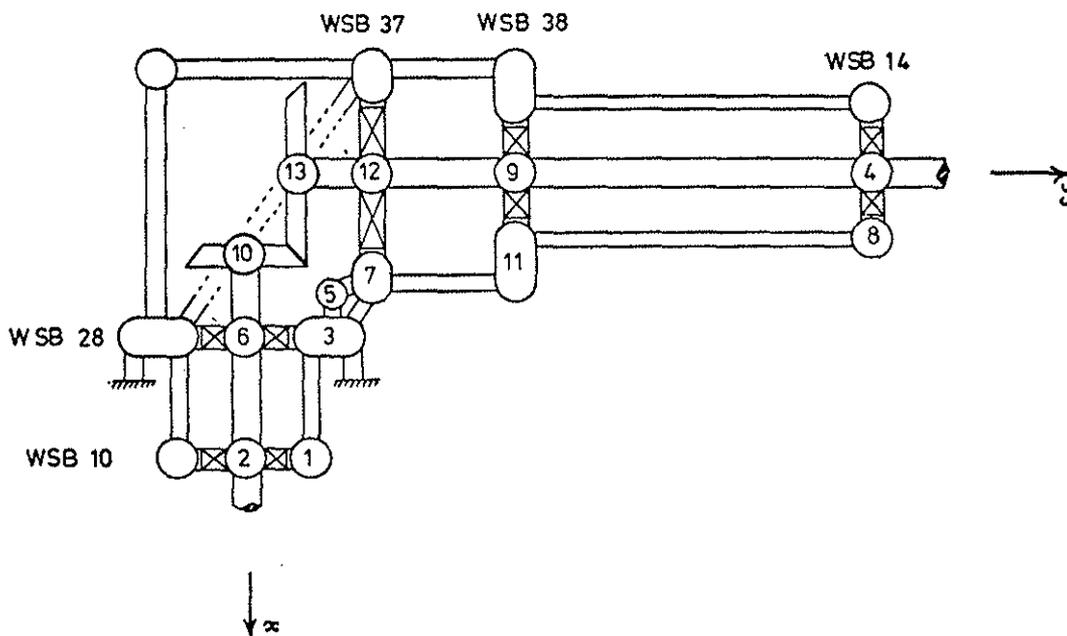
FIGURE 2 MODEL IDEALIZATION AND NODE NUMBERING.
