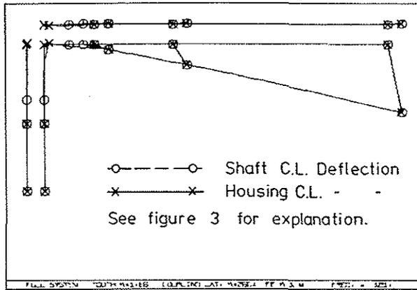
FIGURE 5 PREDICTED MODE SHAPE 121Hz.
