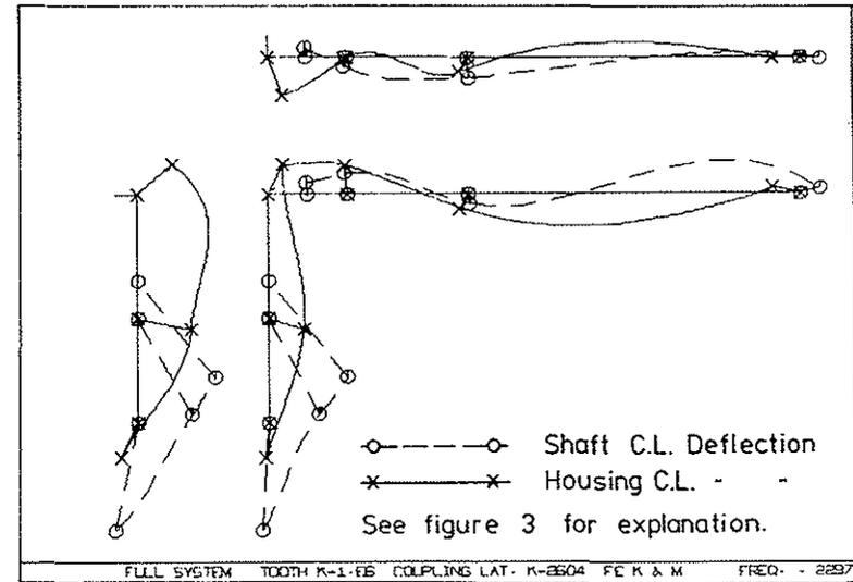
FIGURE 7 PREDICTED MODE SHAPE 2297Hz.
