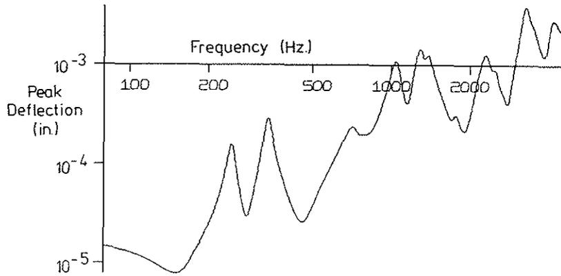
FIGURE 10 FORCED RESPONSE TO .001 IN. NORMAL MESH ERROR NORMAL RELATIVE MESH DISPLACEMENT.
