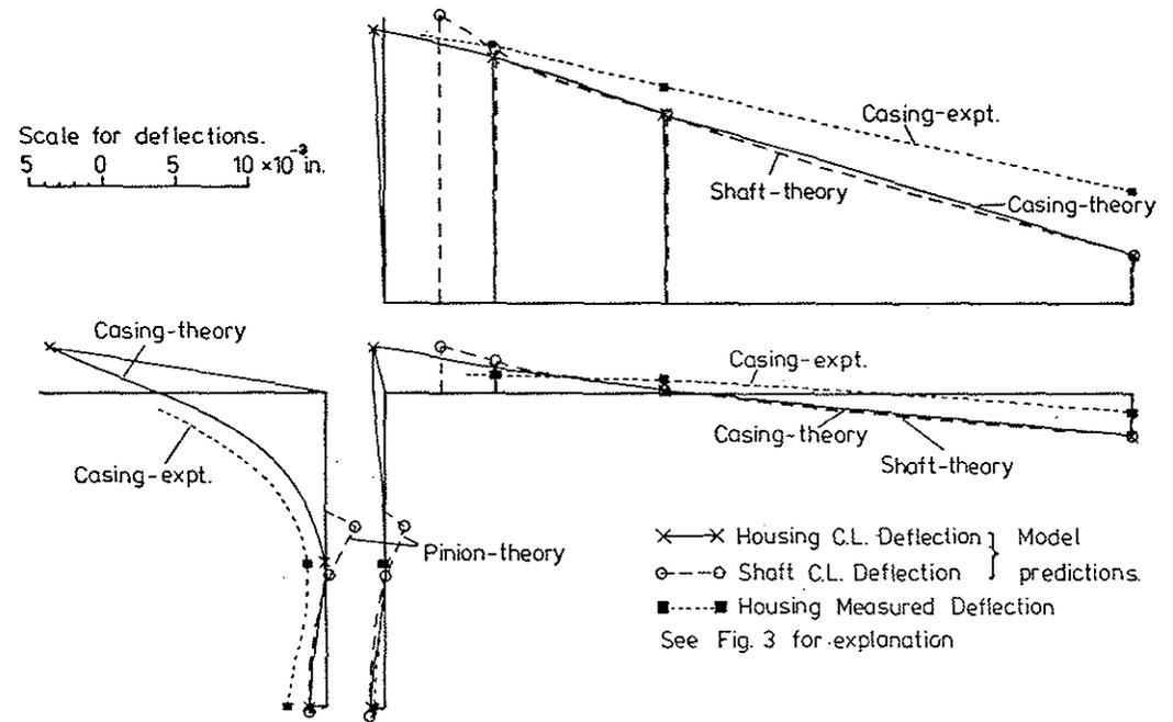
FIGURE 4 PREDICTED AND MEASURED DEFLECTIONS UNDER 4500 LBF-IN TORQUE (1/P).
