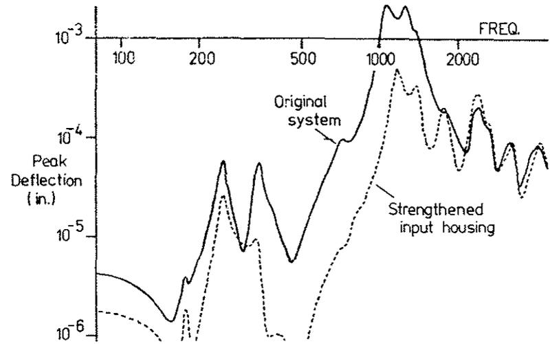
FIGURE 13 FORCED RESPONSE TO .001 IN. NORMAL MESH ERROR ON CASING AT WSB10 OUT OF SHAFT PLANE (1z).
