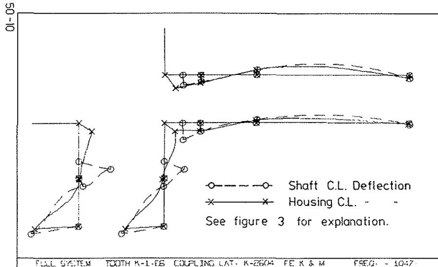
FIGURE 6 PREDICTED MODE SHAPE 1047Hz.
