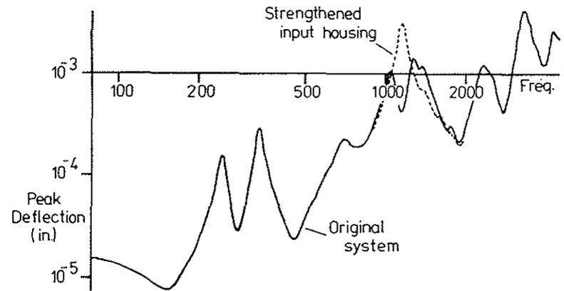
FIGURE 14 FORCED RESPONSE TO .001 IN. NORMAL MESH ERROR NORMAL RELATIVE MESH DISPLACEMENT.
