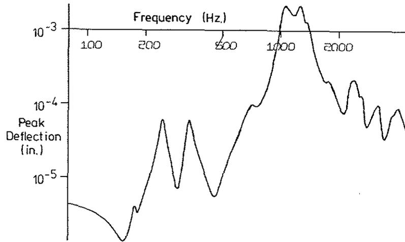
FIGURE 9 FORCED RESPONSE TO .001 IN. NORMAL MESH ERROR ON CASING OUT OF PLANE AT WSB 10 ( $f_z$ )
