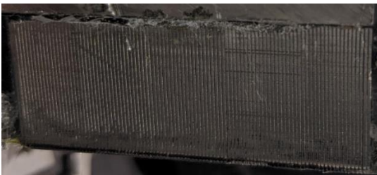
Figure 6: Photo of the electric engine sheet metal stack taken during reverse engineering
