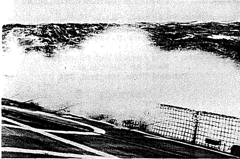
FFG-8 during SH-60B DI Testing
