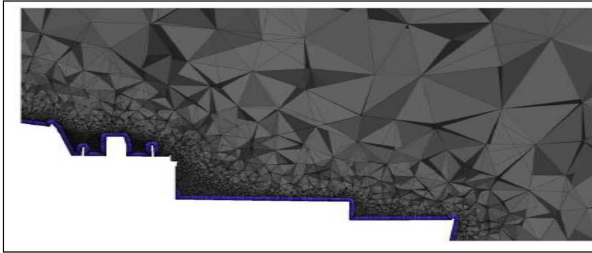
Figure 6. Volumetric mesh visualization on flight deck region.
