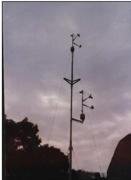
Figure 11 – Gill anemometers at the measurement mast
