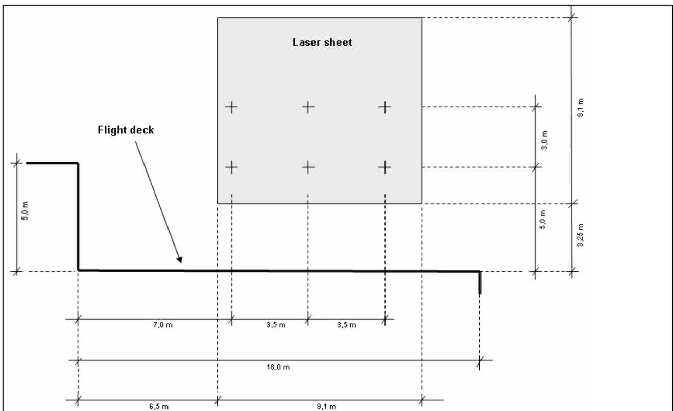
Figure 9 – Laser sheet position and dimension
