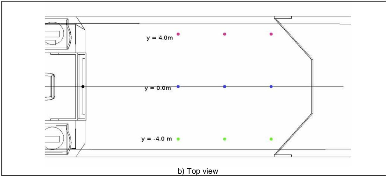
Figure 2 – Position of the anemometers in the *in situ* tests
