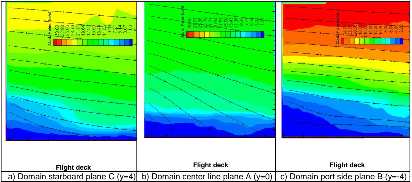
Figure 10 – Wind tunnel results: velocity magnitude [m/s] over the flight deck
