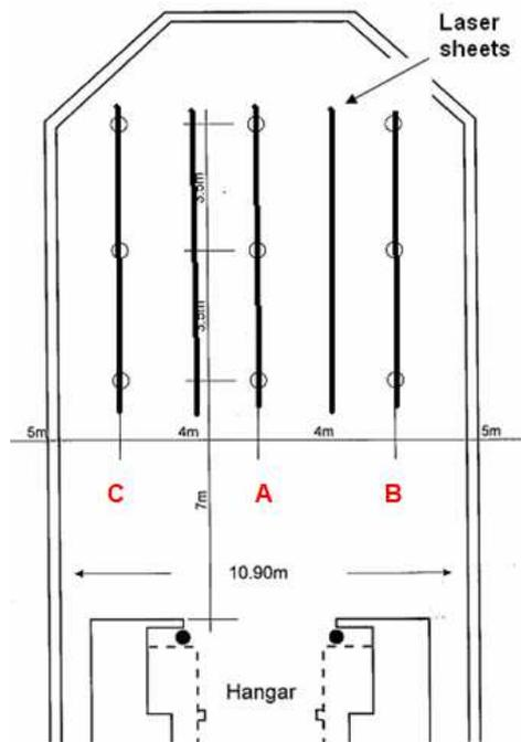
Figure 3 - Schematic representation of the laser sheets in the wind tunnel tests
