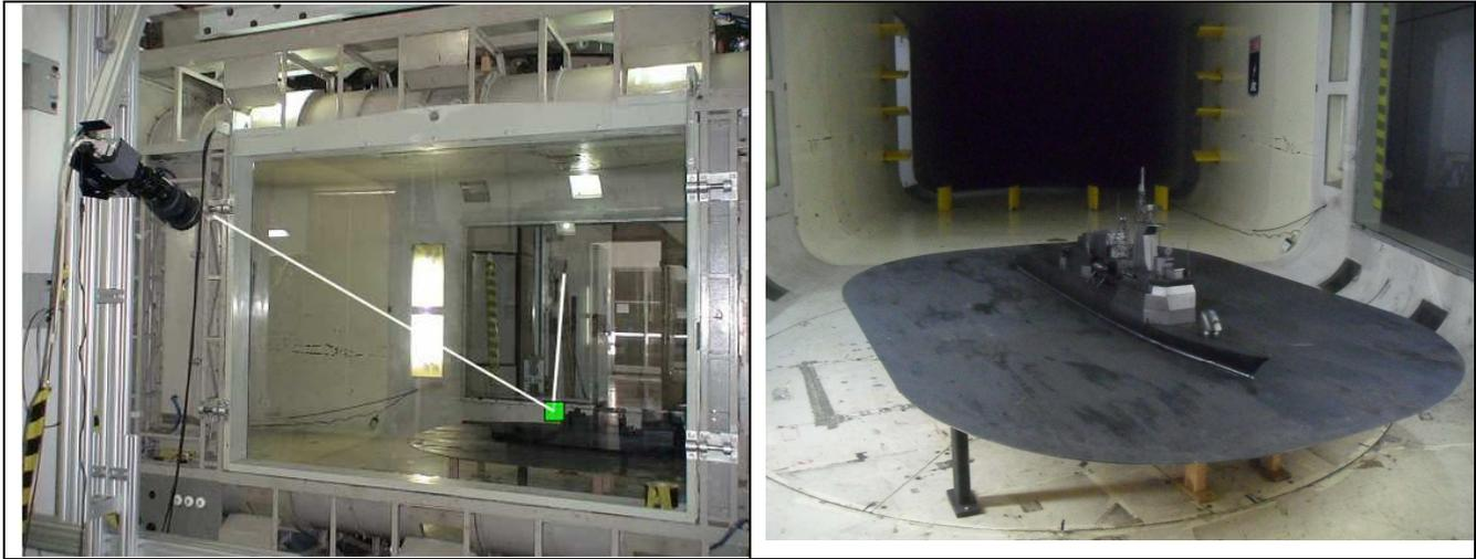
Figure 8 – 1/65 scale model in the IAE wind tunnel
