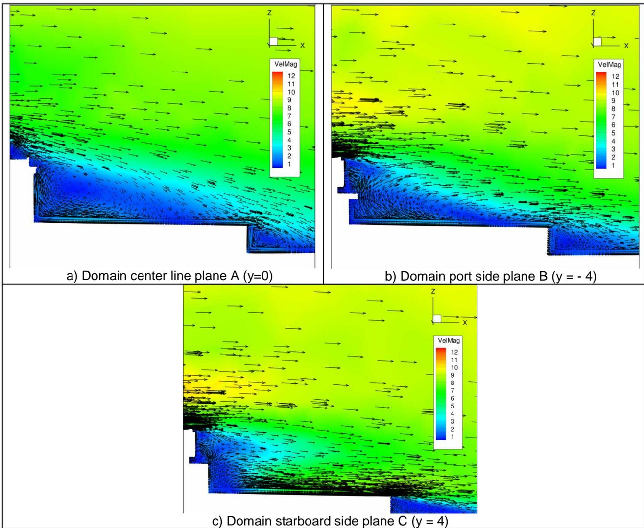
Figure 7. – CFD results: velocity magnitude [m/s] over the flight deck
