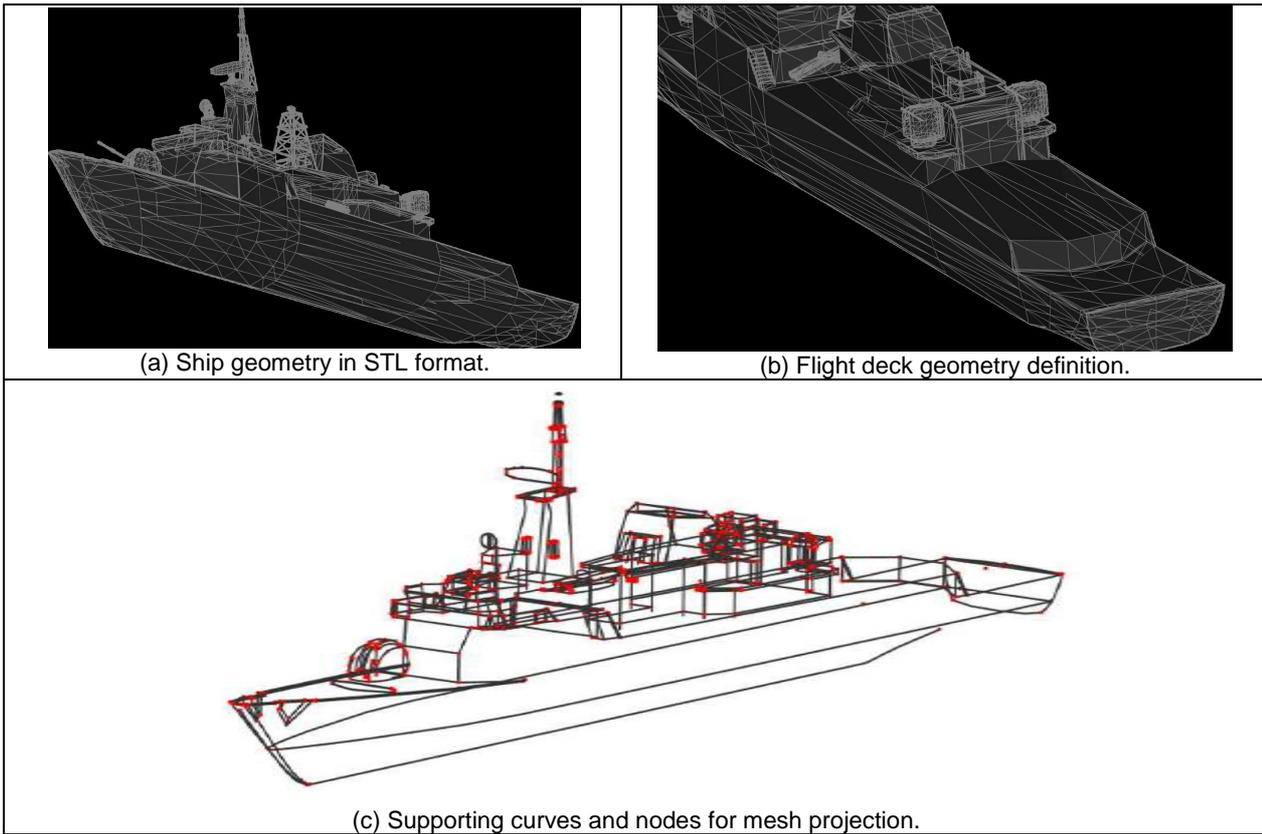
Figure 4. Computational geometry of the Inhaúma-class corvette.
