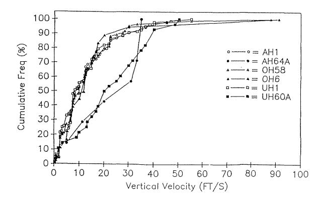
Figure 2. Army Helicopter Vertical Impact Velocity
