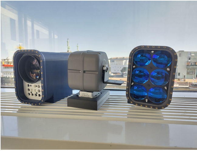
Figure 1. Prototype of the portable range-gating instrument TRAGVIS, originally developed for ship-based applications. The laser illumination module is on the right, the camera/receiver on the left. Both components can be mounted on a motor (middle) enabling pointing the instrument in any direction.
