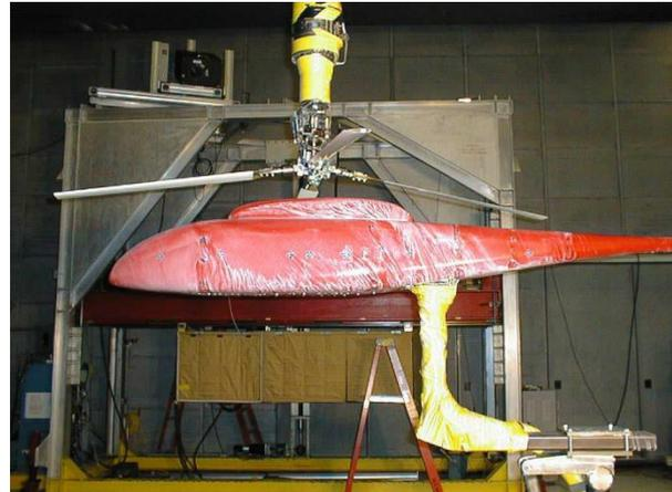
Figure 11: View of the experimental setup of the ROBIN fuselage equipped with a four-bladed rotor.<sup>[17]</sup>
