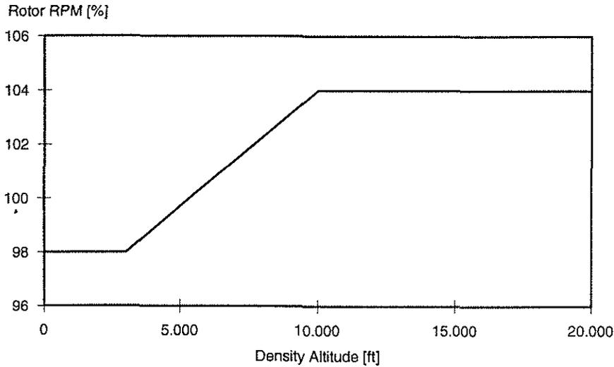
Fig. 22: FADEC controlled variable rotor speed
