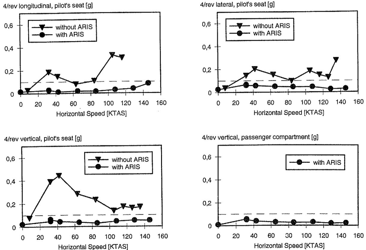
Fig. 17: Vibration level in horizontal flight at pilot's seat and in passenger compartment
