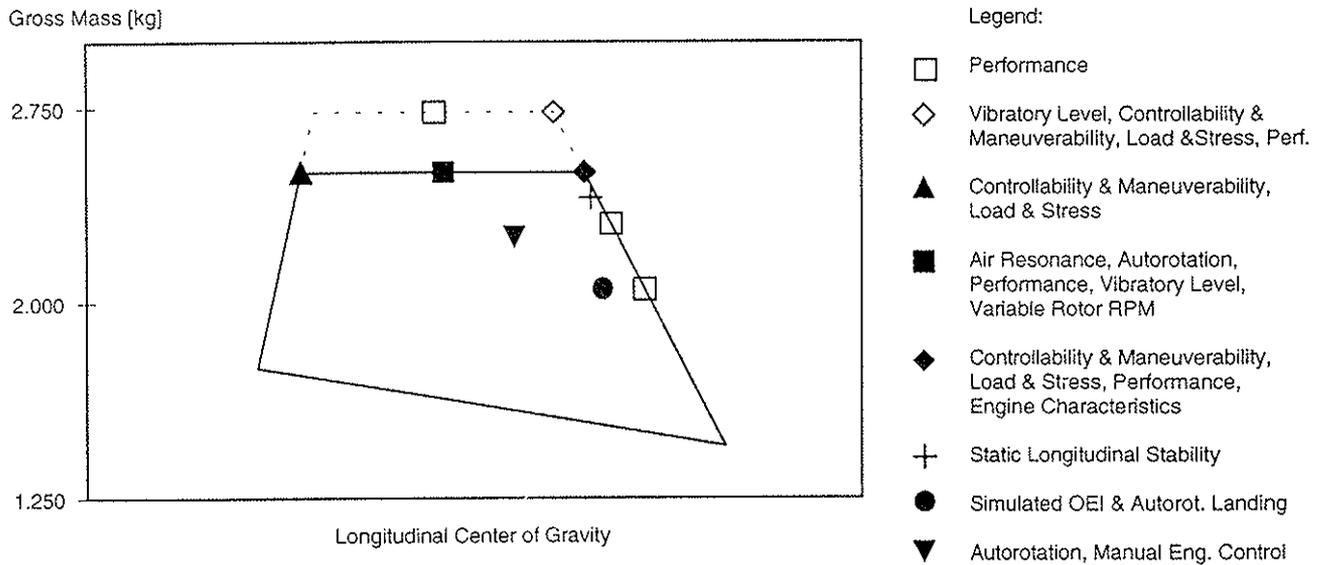
Fig. 4: Center of gravity - overview of tests performed
