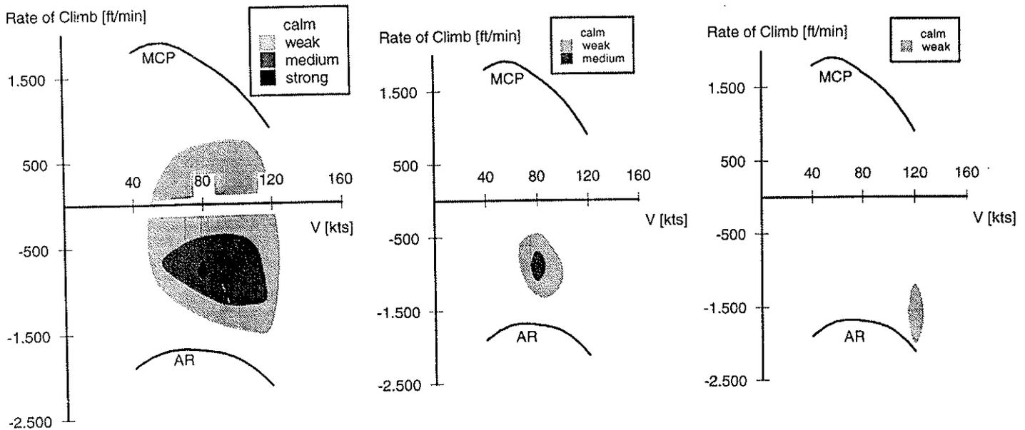
Fig. 16: Tail shake occurrence within the flight envelope
