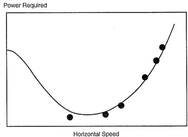
Fig. 9: Level flight power requirement
