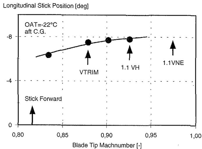
Fig. 11: Static longitudinal stability in horizontal flight
