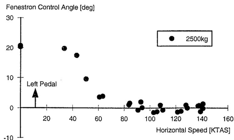
Fig. 18: Fenestron control angle in horizontal flight
