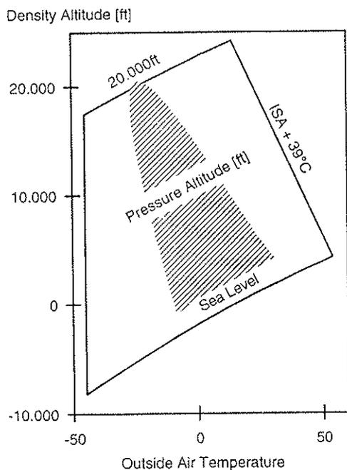
Fig. 5: Flight envelope - tested area
