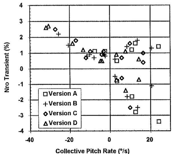
Fig. 20: Nr transient droop vs collective input rate
