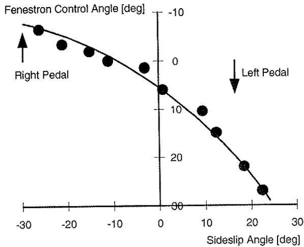
Fig. 12: Directional stability in horizontal flight
