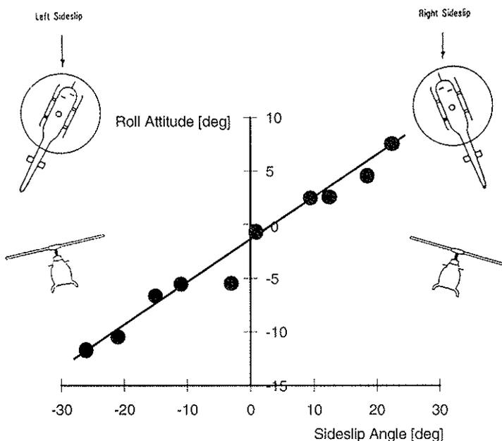
Fig. 14: Sideforce characteristics in horizontal flight
