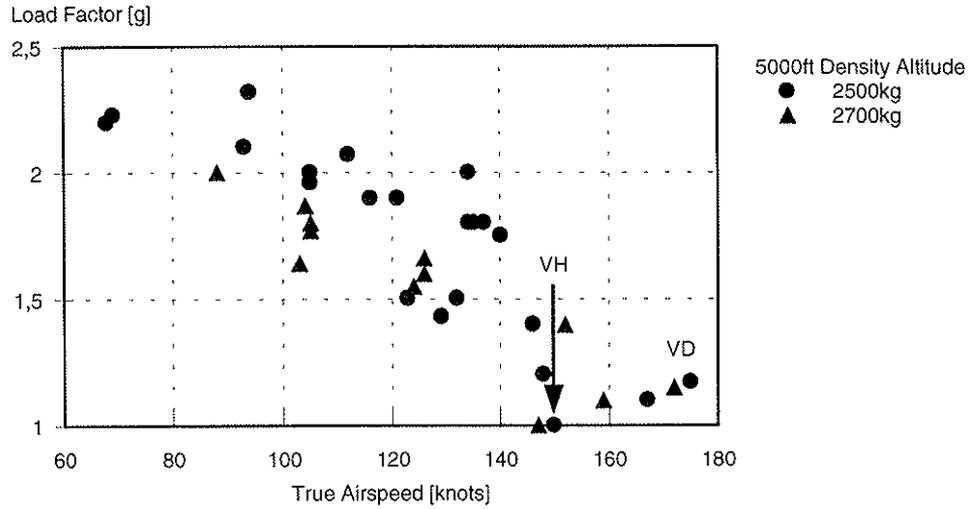
Fig. 15: Normal load factor in forward flight
