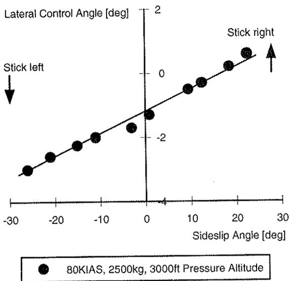
Fig. 13: Dihedral effect in horizontal flight
