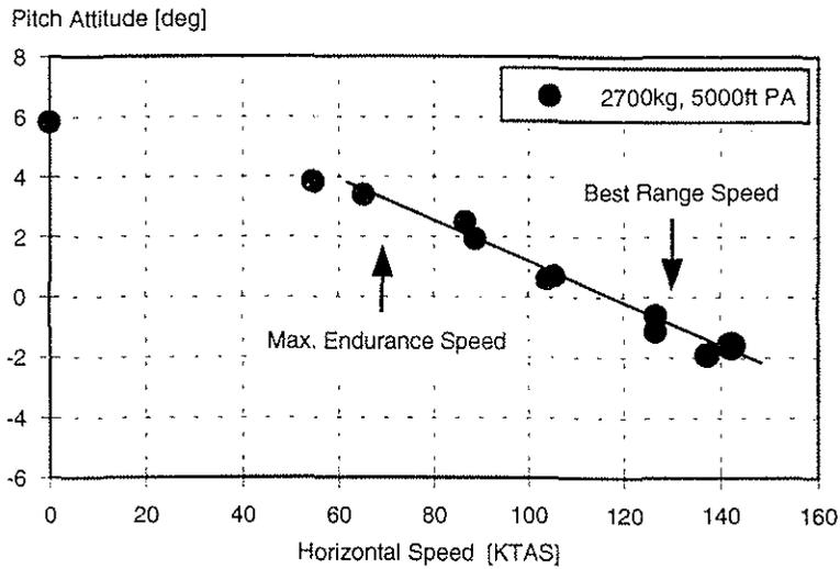
Fig. 10: Pitch attitude in level flight
