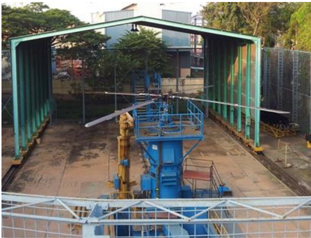
Figure 3: Isolated rotor whirl tower test setup
