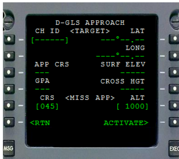
Figure 5: MCDU proposal layout for customized precision approach: CH ID number only data required for autotuning of approach.
