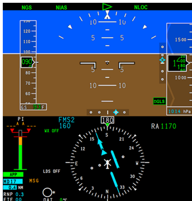
Figure 5: AW189 glass cockpit with lateral/vertical angular deviations in final segment – image for reference only.
