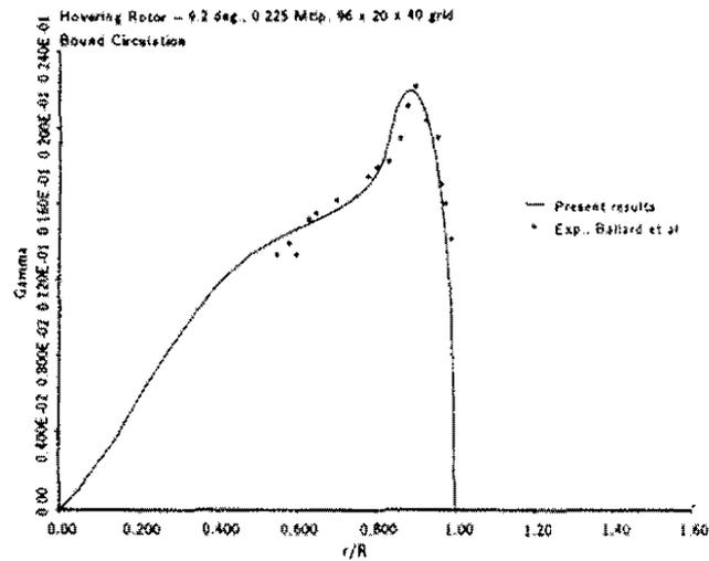
Fig.6 Same as Fig.2 but with bound circulation predicted by Euler solver coupled to FFW geometry .
