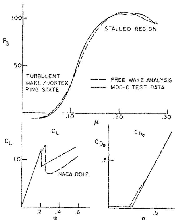
Fig.3 Comparison between measured performance of Mod 0 wind turbine and free wake analysis using lift and drag schedule shown.  $P$  in KW.
