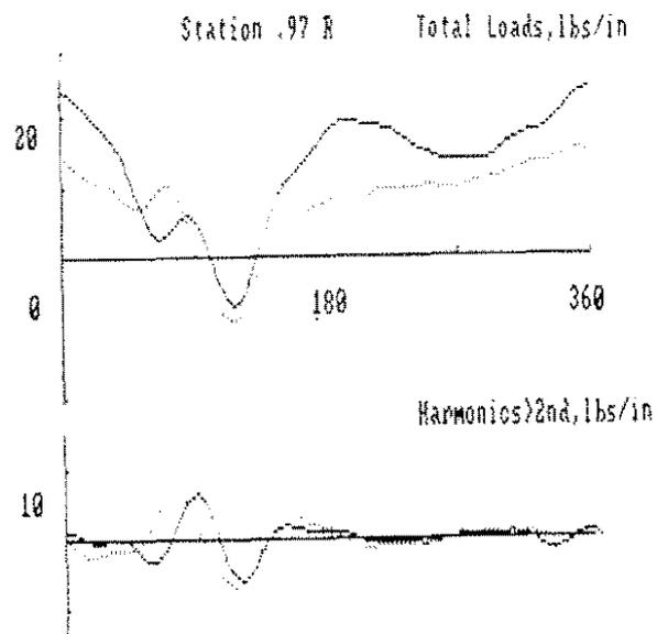
Fig.10 Comparison at 97% span between airloads of Fig.9 with experimental airloads of Fig.7 .
