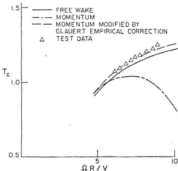
Fig.4 Comparison between predictions of wind turbine thrust coefficients in vortex ring state and wind tunnel tests.
