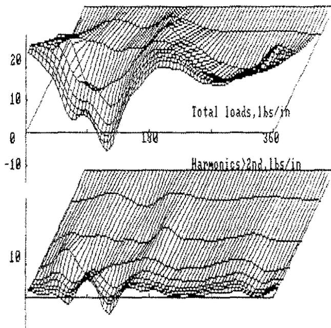
Fig.9 Predicted airloads for same case as Fig.7. Far trailed and shed wakes modeled by rolled up vortex filaments.
