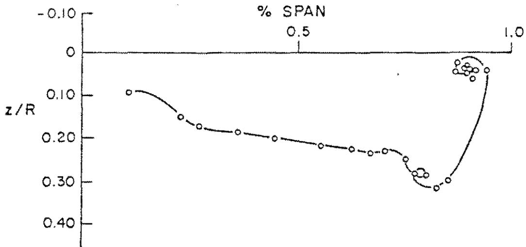
Fig.5 Roll up of complete near wake at 180 deg. azimuth from birth - no far wake effects included.
