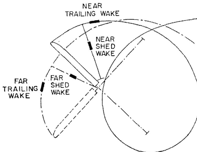
Fig.8 Wake geometry showing near and far trailed and shed wakes.
