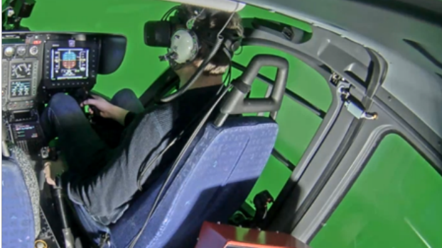
Figure 1: Screenshot of Piloted Campaign in Air Vehicle Simulator (AVES) with Mixed Reality Setup
