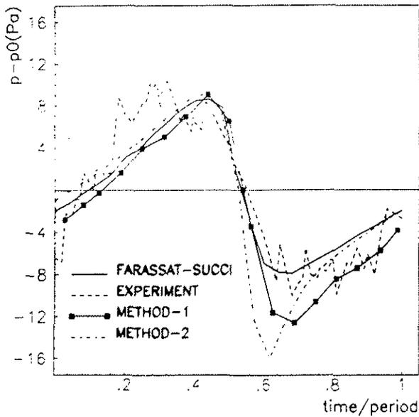
**Figure 1.** Aeroacoustic pressure in the plane of the rotor, at 7.28m from the axis of the rotor, as a function of time. The three-bladed propeller has radius  $R = 1.295m$ , average chord  $c = .1538m$ , and non-linear twist varying from  $50^\circ$  at the root to  $23^\circ$  at the tip. The tip Mach number is  $M_{TIP} = .71$ , corresponding to a rotational speed of 1,760rpm.
