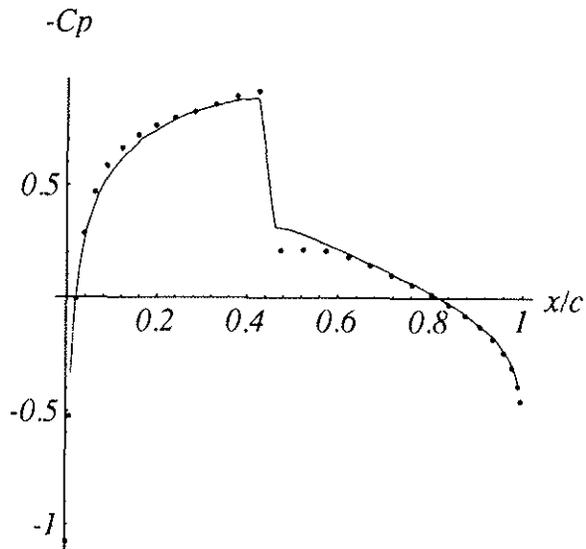
**Figure 4.** Pressure coefficient along the chord for the same case of Fig.1. The result of the formulation from Eq. 20 (dots) is compared to the results of Ref. [9].
