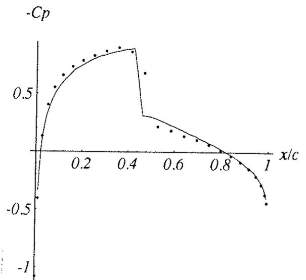
**Figure 6.** Pressure coefficient along the chord for the same case of Fig.3. The result of the formulation from Eq. 24 (dots) is compared to the results of Ref. [9].
