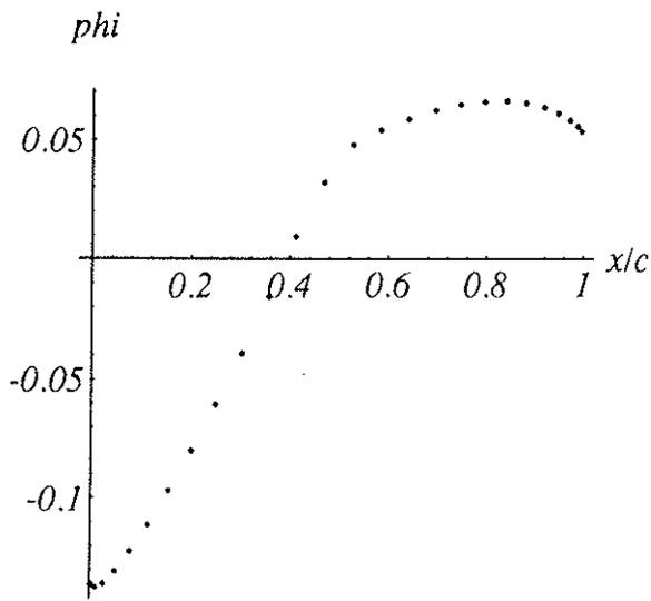
**Figure 5.** Velocity potential distribution in transonic regime. NACA 0012 airfoil, incidence  $\alpha = 0^\circ$ , free stream mach number  $M_\infty = 0.8$ . Nonlinear term from Eq. 24.
