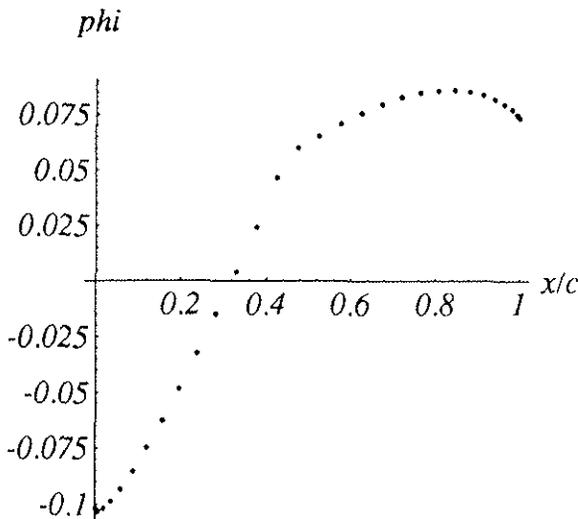
**Figure 3.** Velocity potential distribution in transonic regime. NACA 0012 airfoil, incidence  $\alpha = 0^\circ$ , free stream mach number  $M_\infty = 0.8$ . Nonlinear term from Eq. 20.
