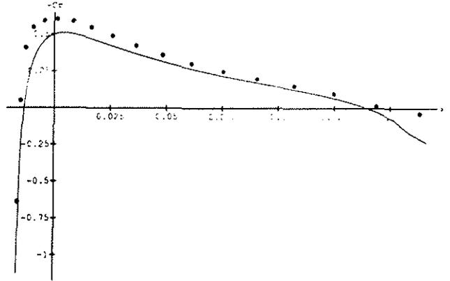
**Figure 2.** Non-lifting rotor in transonic range. Chordwise pressure distribution at the tip section for a monoblade rotor.  $M_{TIP} = 0.830$ ,  $\theta_c = 0^\circ$ . Present analysis (dotted line) is compared to the results of a FDM code [22], (solid line).
