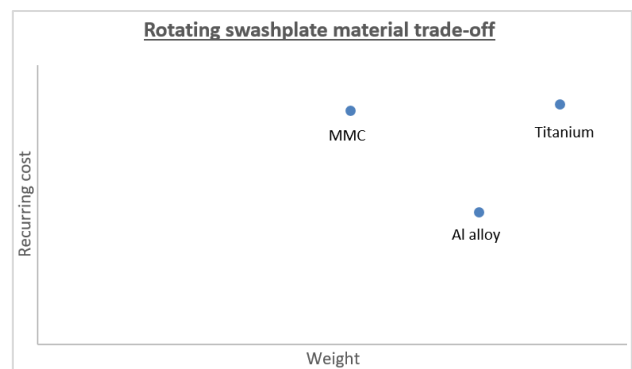
Figure 21 – Material trade-off for swashplate
