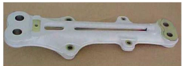
Figure 17 –Main rotor sleeve in MMC
