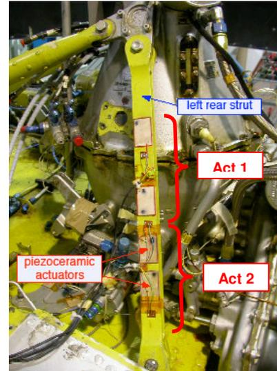
(b) Left rear strut actuators configuration
