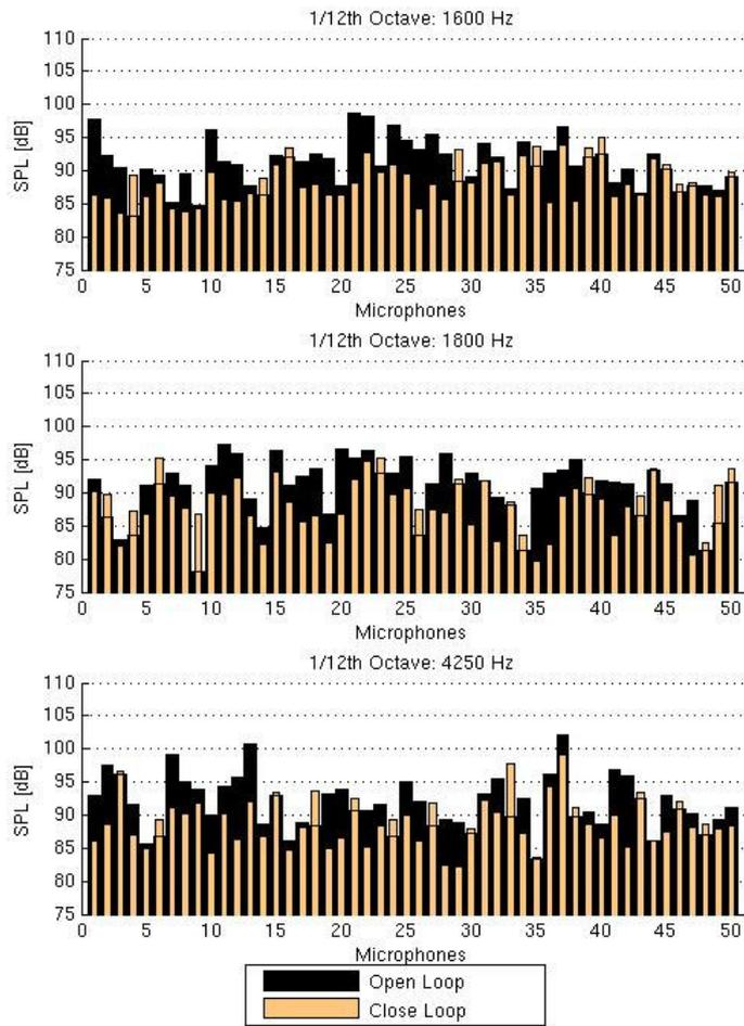
fig. 7 FXLMS: acoustic performance on the 50 measurement points on the three controlled tones
