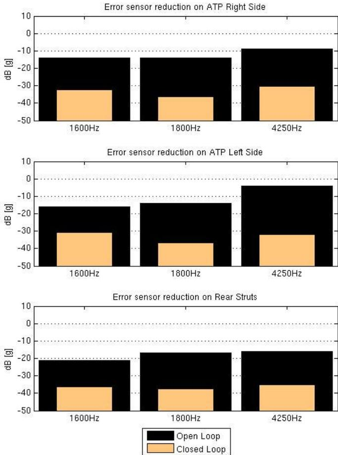
fig. 6 Error sensor vibration reduction respectively on anti-torque plate and struts: dark bar are measured in open loop and clear bar in closed loop.
