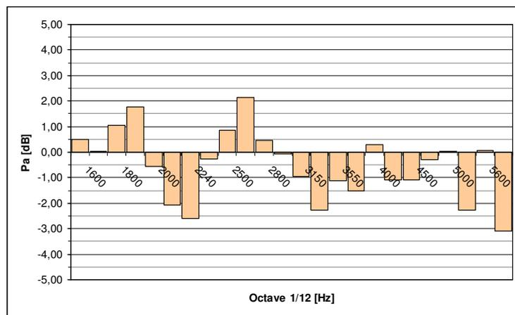
fig. 11 SPL variation passing from 0.8 Kg to 1.5 Kg in 1/12<sup>th</sup> octave band
