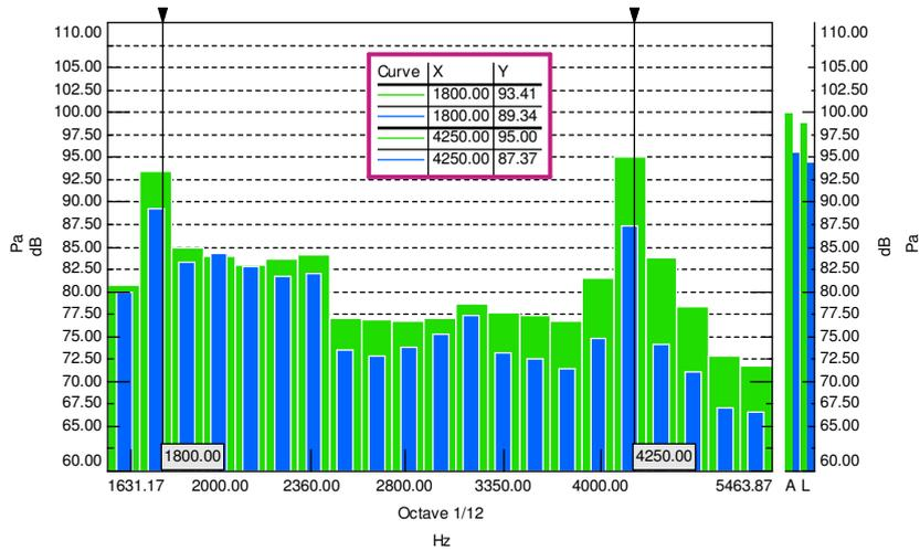
fig. 10 Mean SPL regulation with 4 masses of 1500 grams: green bar without mass, blue bar with mass on anti-torque plate bolts
