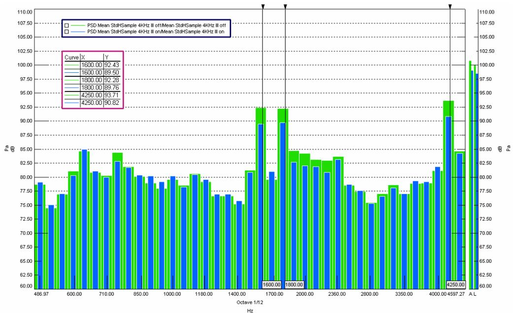
fig. 8 Mean SPL regulation measured on 50 microphones: green bar in open loop, blue bar in closed loop
