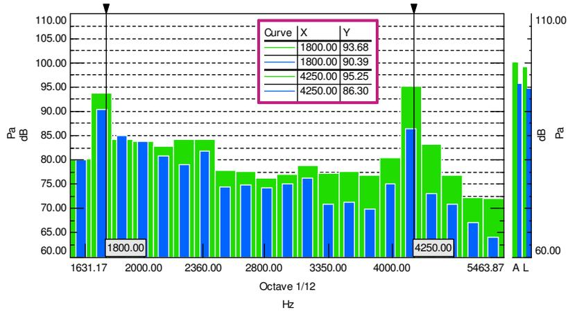
fig. 9 Mean SPL regulation with 4 masses of 800 grams: green bar without mass, blue bar with mass on anti-torque plate bolts
