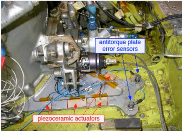
(a) Anti-torque plate actuators/sensors configuration
