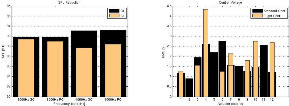
(a) Comparison between SPL reduction (mean on 50 measurement points) inside cabin in standard configuration (SC) and reduced configuration (FC)
