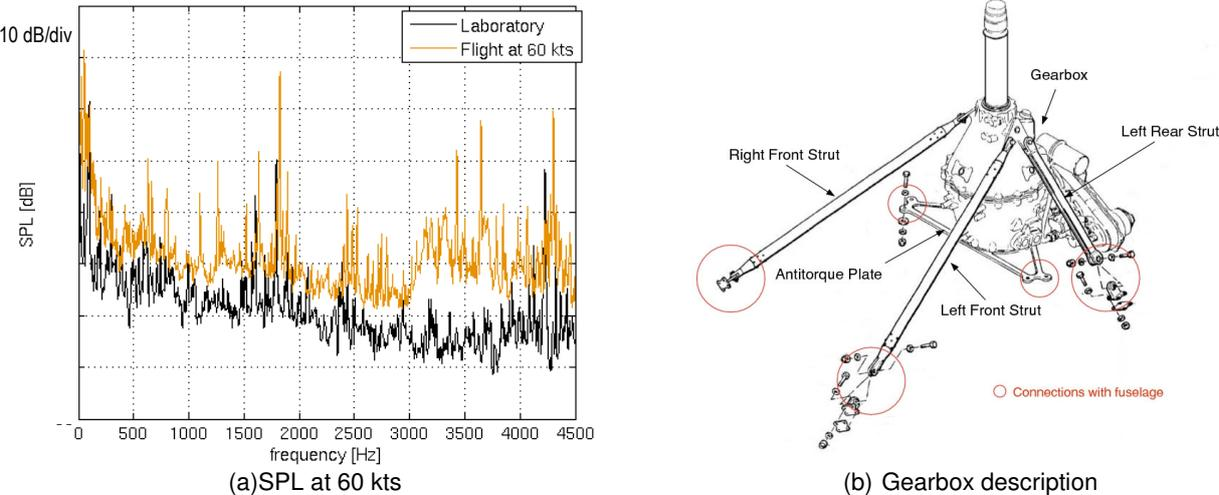
fig. 2 In-flight and laboratory spectrum and gearbox description
