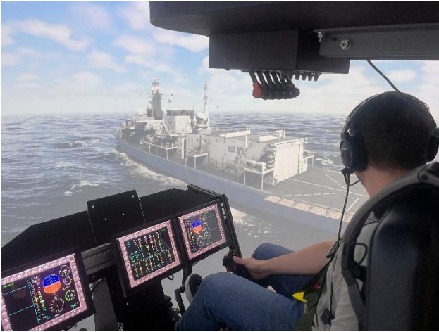
Figure 20: HELIFLIGHT-R visual environment for piloted SHOL assessment
