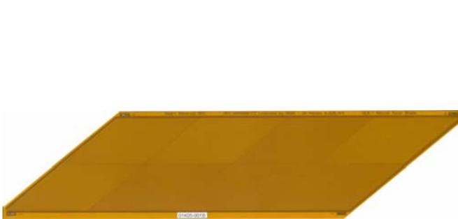
Figure 3: special shaped MFC actuators; height 60,2mm; width 222mm
