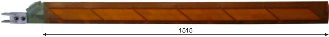
Figure 4: top view of the active twist blade
