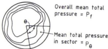
Figure 5: Illustration of total-pressure contours and  $\theta$  sector for definition of distortion coefficient [5].
