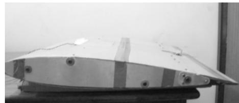
**Figure 5.** Side view of physical model of the wing section
