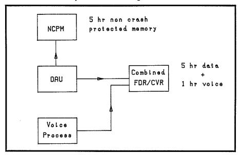
Fig.9 Combined Voice and Data Recorder System
