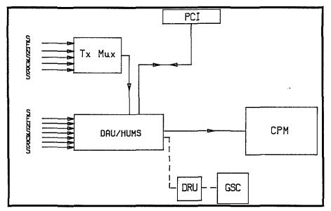
Fig.12 Fully Integrated FDR/HUM System
