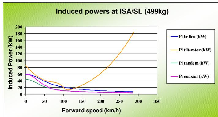
**Figure 12 :** Comparisons of the induced powers for the coaxial and the equivalent helicopter, tandem, tilt-rotor.
