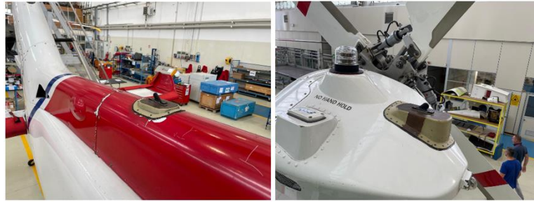
Figure 17 – Antenna 1 and Antenna 2 (TOP) installation
