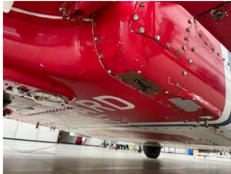
Figure 18 – Antenna 3 and Antenna 4 (BOTTOM) installation
