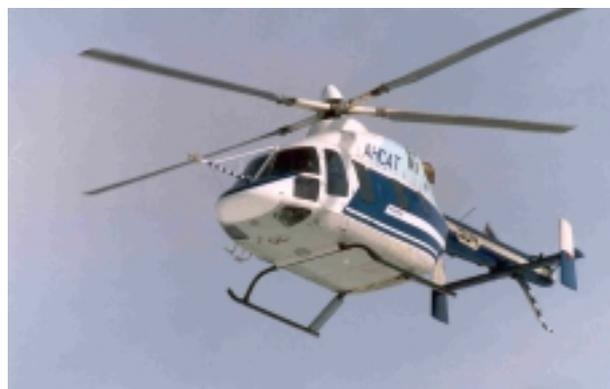
Fig.1. "Ansat" light multi-purpose helicopter
