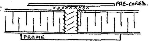
4.9. Panel edge electroless copper plated and butt strap co-cured. Plating slightly inferior to Method 4.8.
