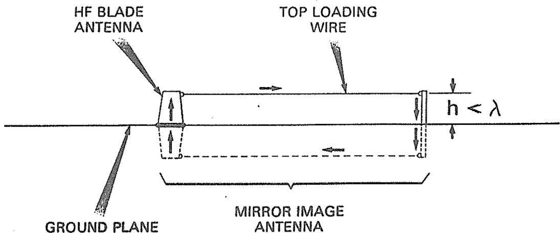
Thus the impedance of this system would be that of an open circuit resonant transmission line of 29 ins spacing, using single core 0.051 inch diameter cable.
