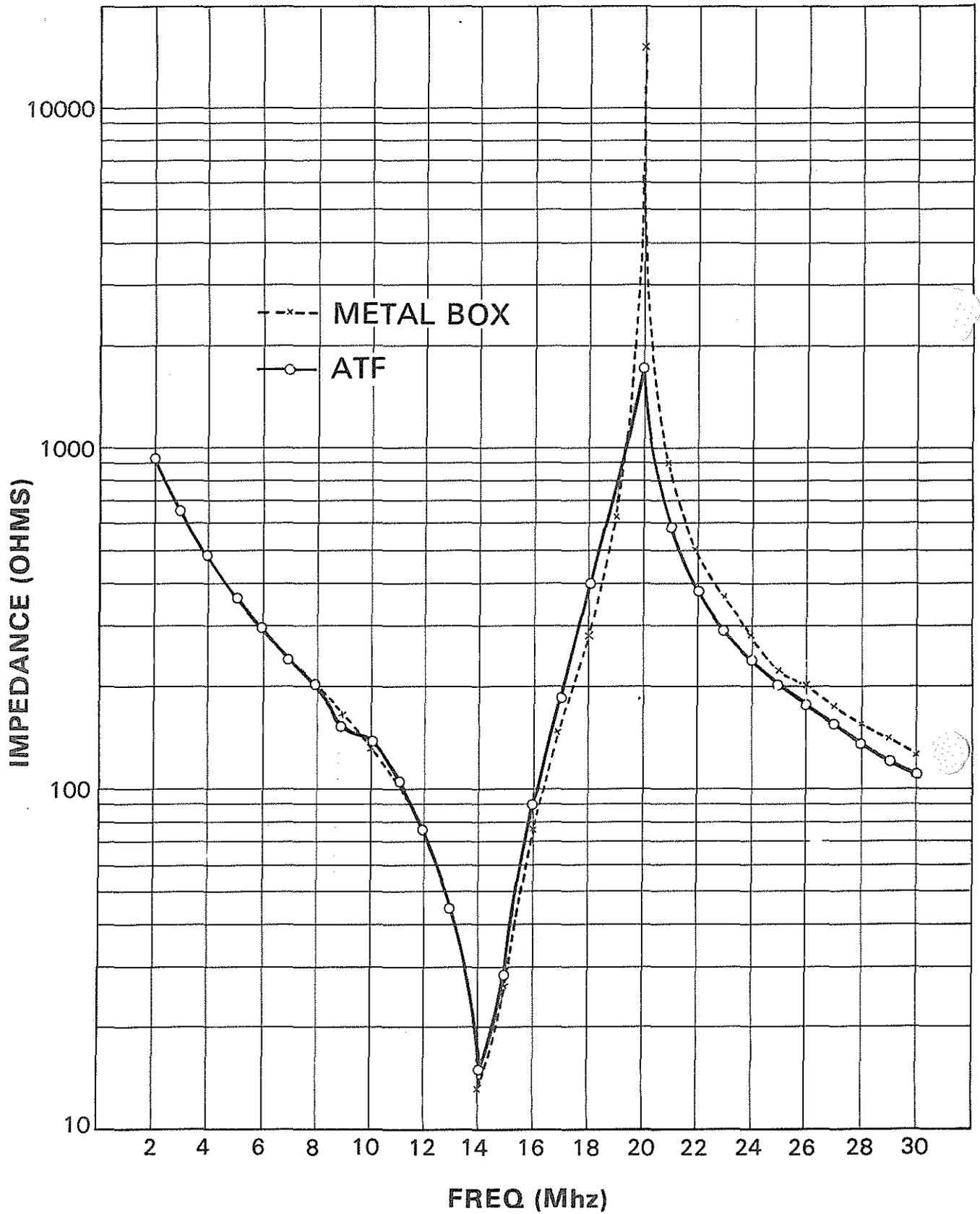
The introduction of losses into the line system has the effect of reducing the impedance peaks from infinity under lossless conditions, and in all practical cases the impedance will be finite, but the extent to which the impedance is reduced is determined by the system loss.
