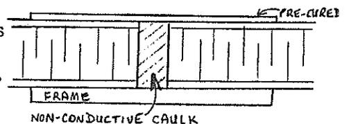
\* Co-cured: Application of uncured prepreg materials with no adhesive layer present. Bond strength derived from resin present in prepreg.
