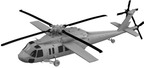
Figure 1: Impression of the compound version of the Black Hawk helicopter (Image adapted from: [11])
