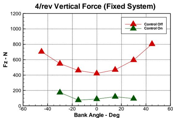
Fig.22: 4/rev hub loads in manoeuvre flights at 80 kts
