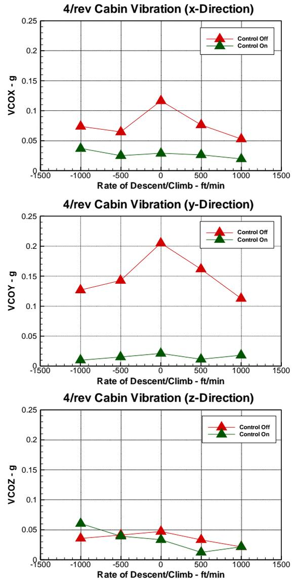
Fig.21:4/rev cabin vibration vs. rate of climb/descent at 65 kts
