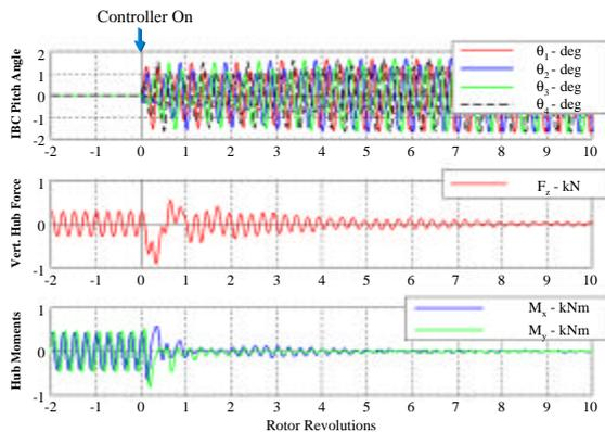
Fig. 11: Simulation of vibration controller activation
