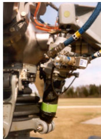
Fig. 3: Servo-hydraulic actuator
