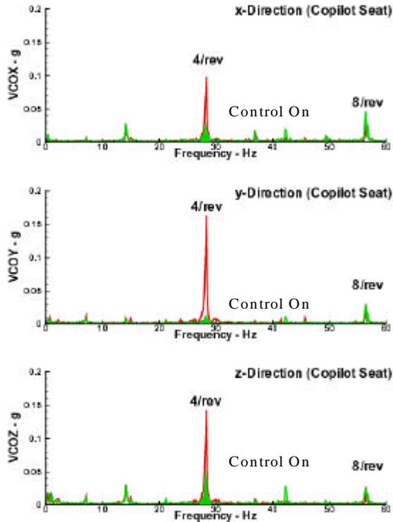
Fig. 26: IBC vibration reduction achievements (BO105 S1 @ 60kts level flight)
