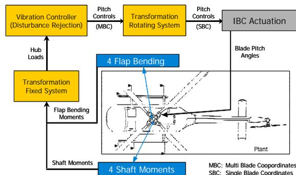
Fig. 10 Schematic view of the vibration control system
