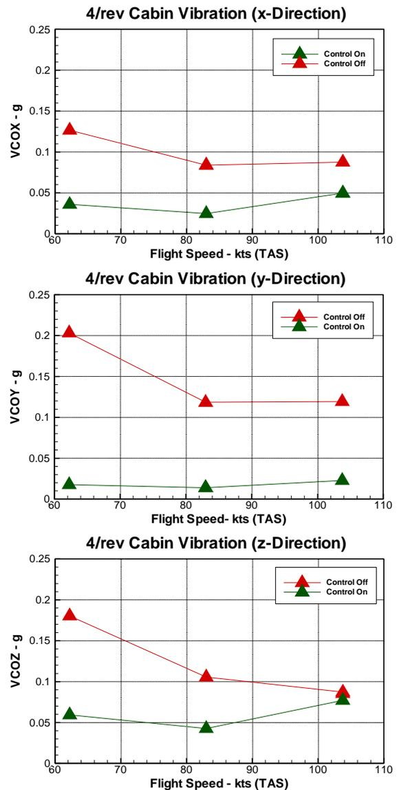
Fig. 19: 4/rev cabin vibration vs. flight speed (100% rotor speed)
