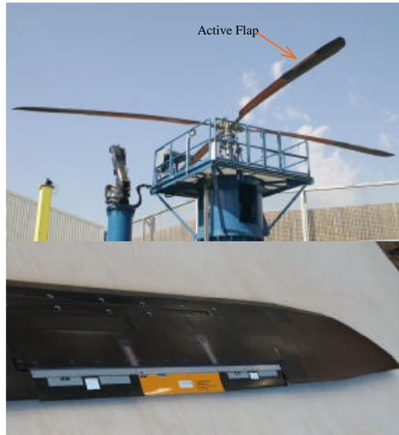
Fig. 27: Experimental main rotor with piezo-active trailing edge flaps on whirl tower
