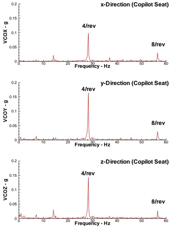
Fig. 2 BO105 S1 vibrations in level flight @ 60 kts
