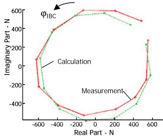
Fig. 13: Comparison of 4/rev vertical forces (Fz) at 100 kts (calculation vs. measurement)
