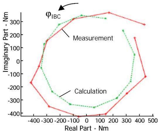
Fig. 15: Comparison of 4/rev pitch moments ( $M_y$ ) at 100 kts (calculation vs. measurement)
