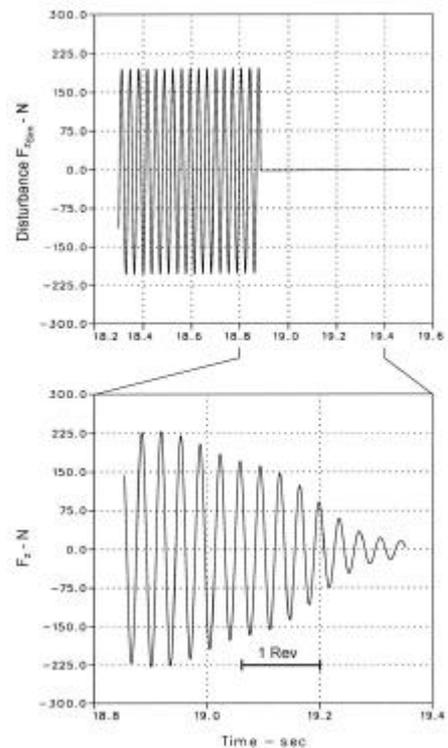
Fig. 25: Evaluation of stability margins from transients ( $F_z$  – control)
