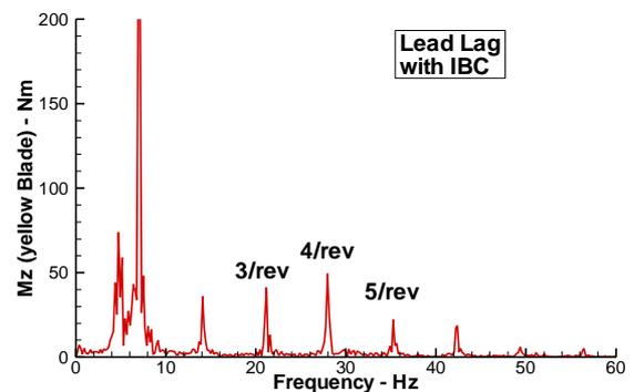
Fig.24: Amplitude spectrum of  $M_x$  with IBC
