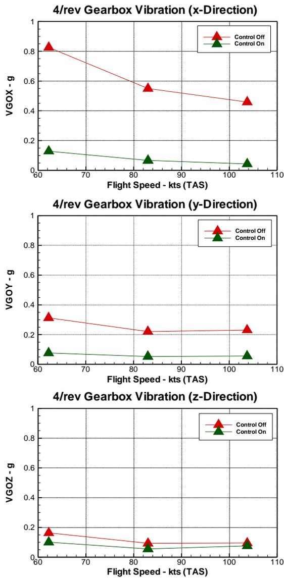
Fig. 18: 4/rev gearbox vibration vs. flight speed (100% rotor speed)
