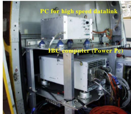
Fig. 4 Integration of the IBC computer and the data acquisition system into the helicopter
