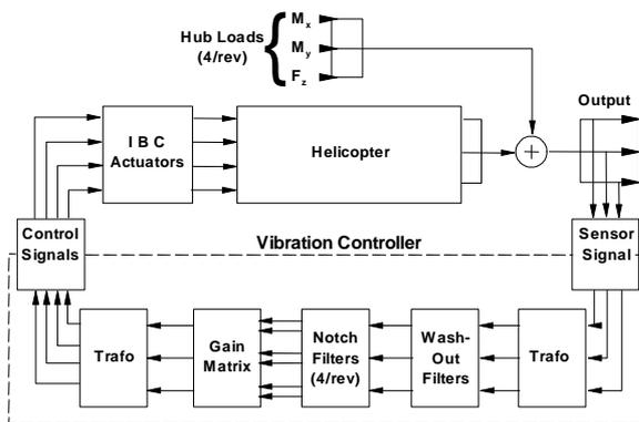
Fig. 7: Feedback loop for 4/rev hub load disturbance rejection (fixed system)
