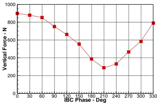
Fig. 12: Vertical hub force in dependence of the IBC phase in level flight (100kts)
