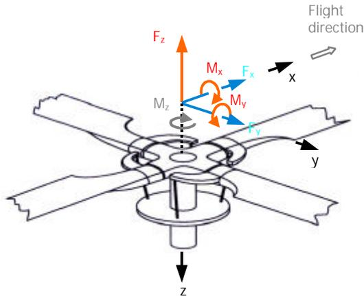
Fig. 6: Hub loads for feedback control
