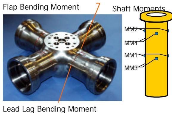
Fig 8: Sensors in the rotating system
