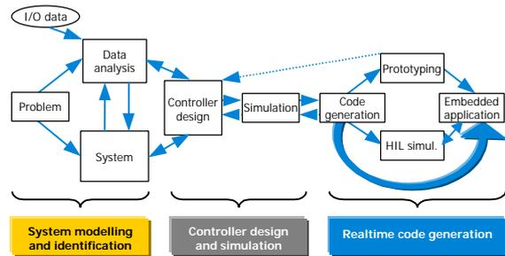
Fig. 9: Realtime controller realisation
