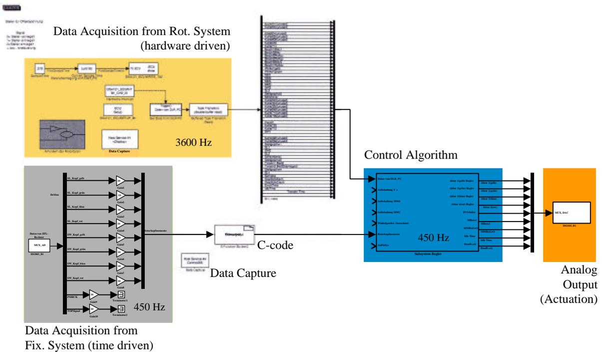
Fig A2: Top level Simulink model of the vibration controller
