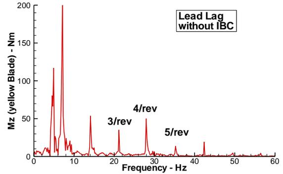
Fig.23: Amplitude spectrum of  $M_x$  without IBC
