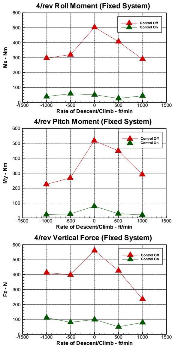
Fig 20: 4/rev hub loads vs. rate of climb/descent at 65 kts
