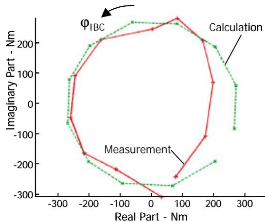
Fig. 14: Comparison of 4/rev roll moments (Mx) at 100 kts (calculation vs. measurement)
