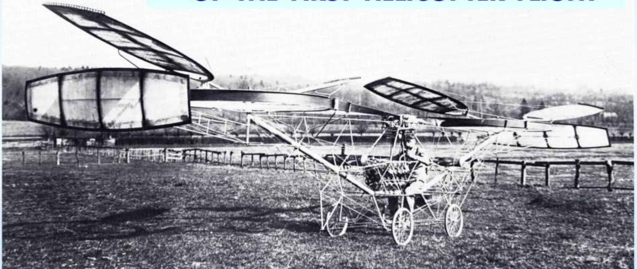
CORNU's helicopter which achieved the first true free flight November 13, 1907
