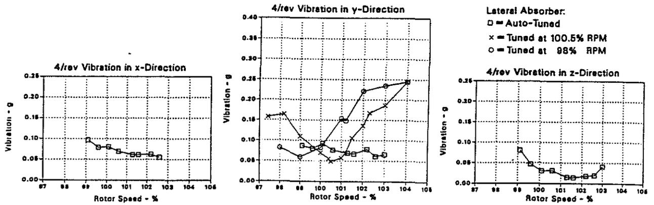
Fig. 15: EC135 Vibration at Pilot Seat (RPM Range at 120 KIAS Level Flight)
