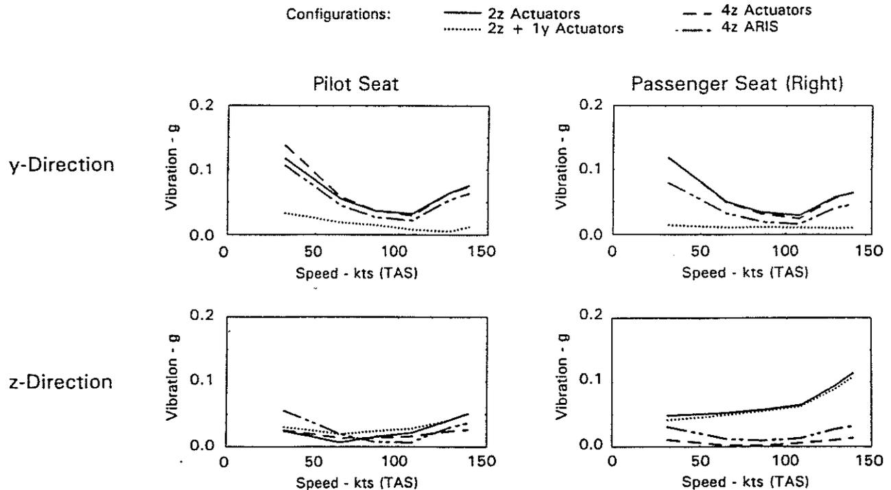
Fig. 20: Potential of ACSR Configurations for Vibration Reduction (EC135): 4/rev Cabin Vibrations
