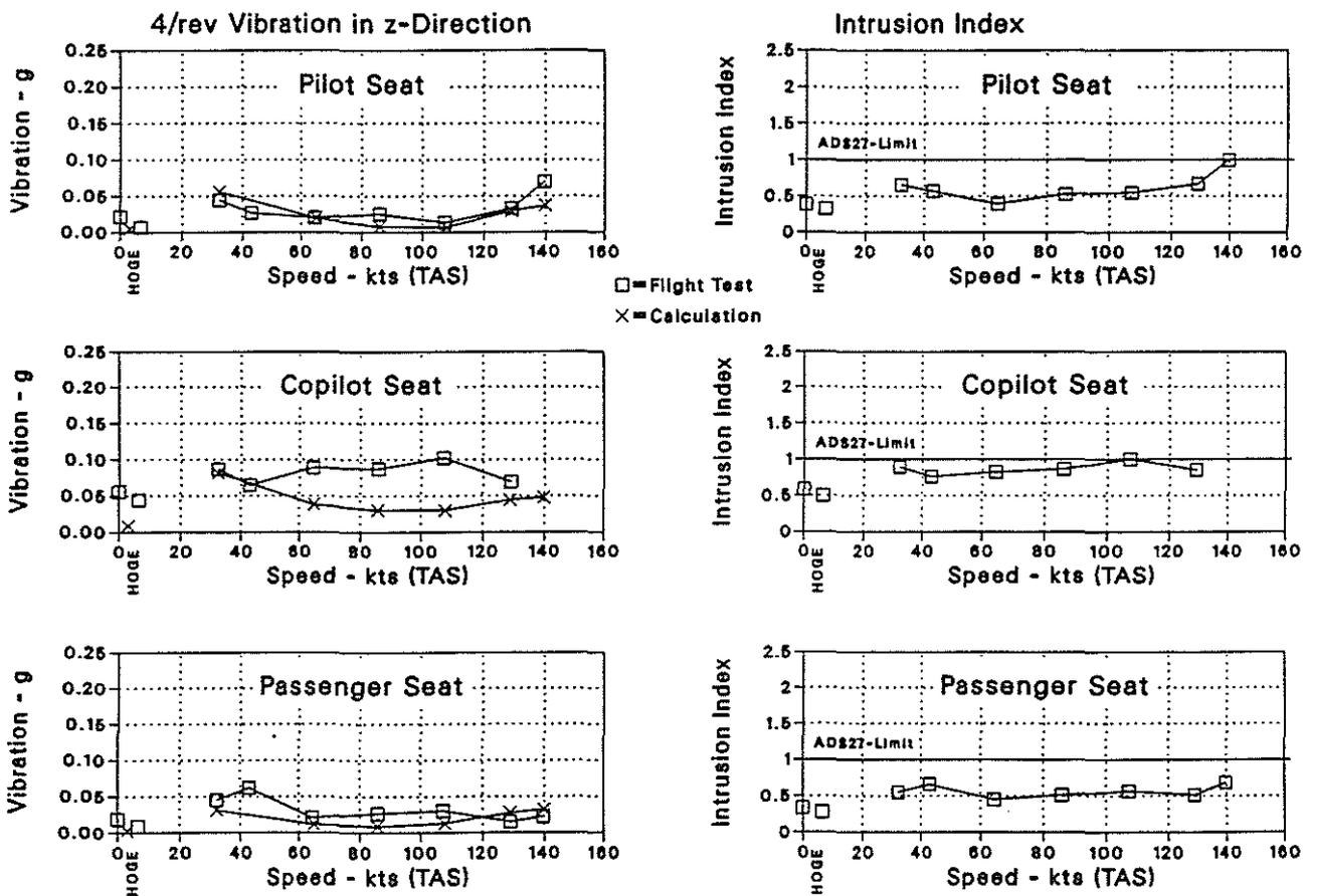
Fig. 16: EC135 Vibration Characteristics (Level Flight)
