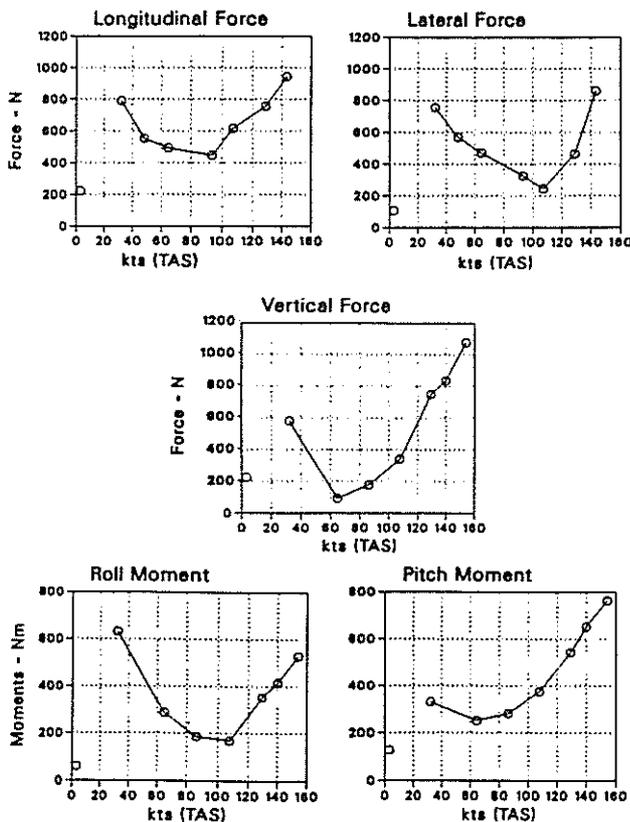
Fig. 12: EC135 Vibratory 4/rev Hub Loads (Level Flight)
