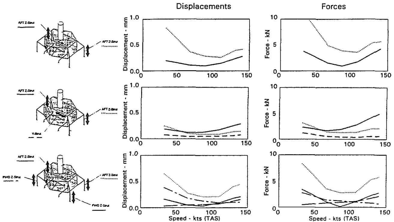
Fig. 21: Requirements of ACSR Configurations for Piezo Actuators (EC135)
