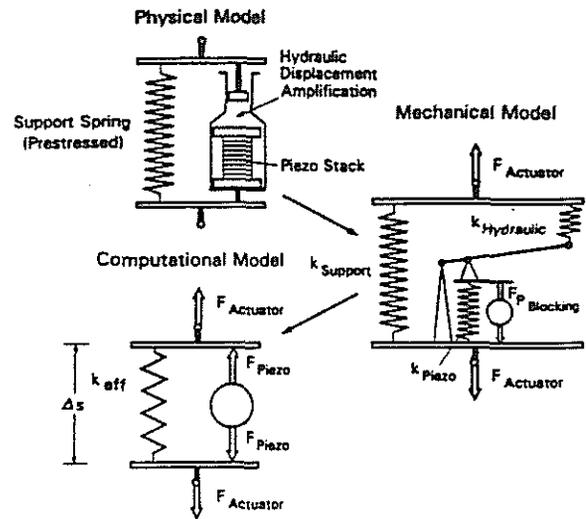
Fig. 22: Piezo Actuator with Hydraulic Displacement Amplification
