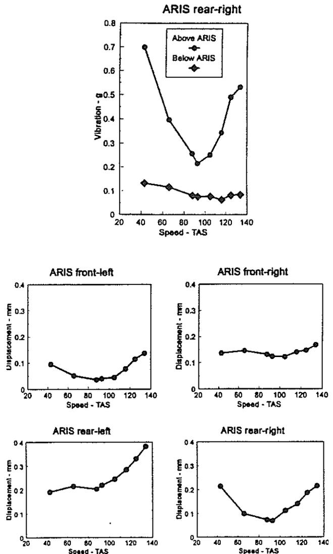
Fig. 13: EC135 ARIS Measurements (Level Flight) 4/rev Displacements and Attachment Vibrations
