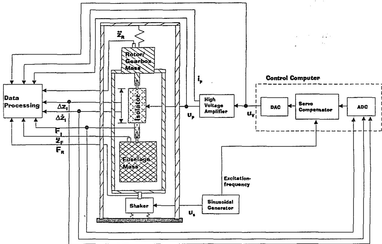
Note: Isolator force  $F_i$  measured by load cell or fuselage accelerometer (indirect)
