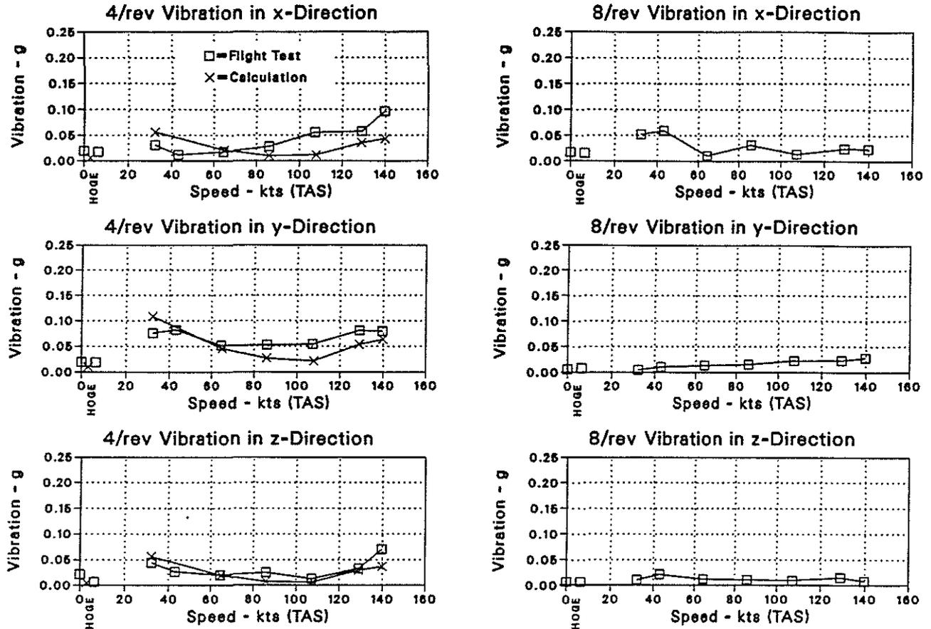
Fig. 14: EC135 Vibrations at Pilot Seat (Level Flight)
