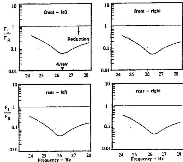
Fig. 8: EC135 Isolator Transmissibilities (Test Rig Results)
