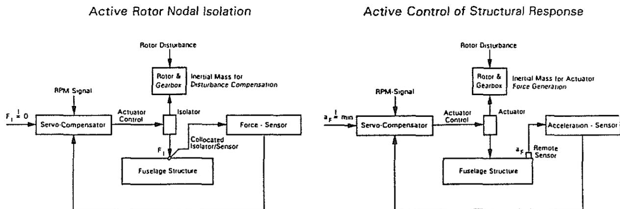
Fig. 17: Active Vibration Control Concepts - Nodal Isolation vs. ACSR
