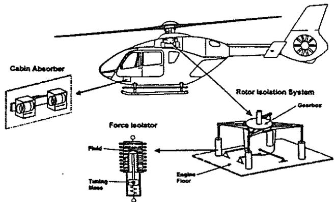
Fig. 3: EC135 Vibration Control Means
