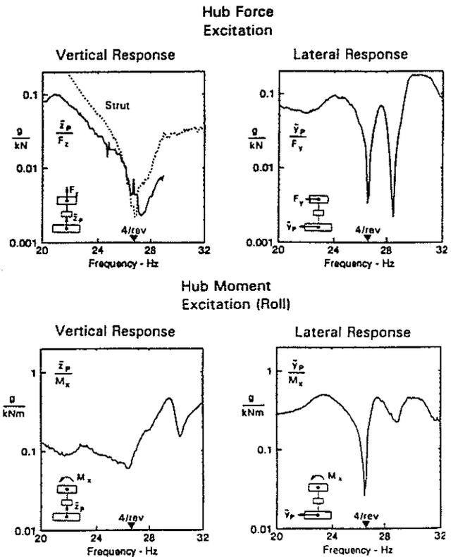
Fig. 11: EC135 Acceleration Transmissibilities at Pilot Seat (Shake Test Results)
