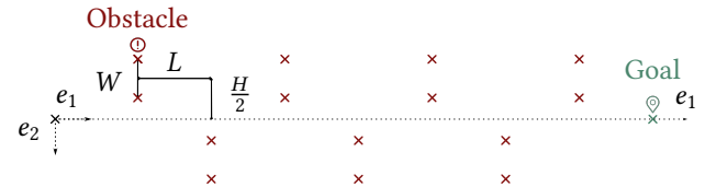
Fig. 3: Definition of geometrical quantities defining task of slalom
