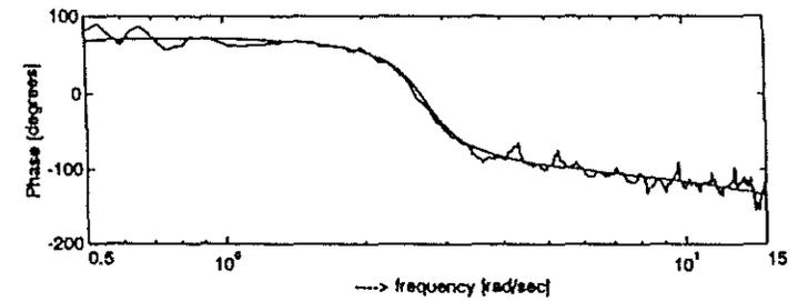
Fig 4: Comparison of BO-105 flight data and identified frequency response - dped to r
