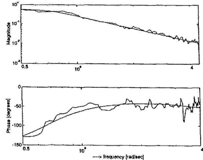
Fig 5: Comparison of BO-105 flight data and identified frequency response - dlon to u
