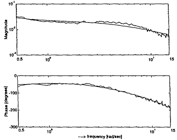
Fig 2: Comparison of BO-105 flight data and identified frequency response - dlon to q
