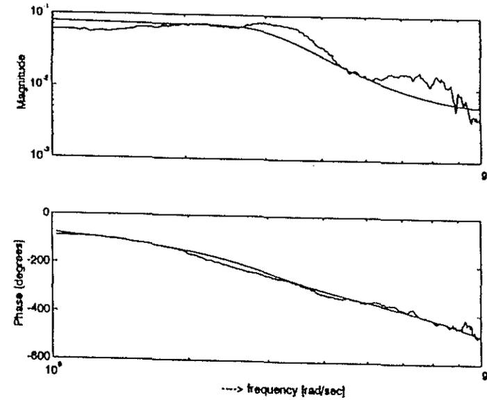
Fig 6: Comparison of BO-105 flight data and identified frequency response - dlat to v
