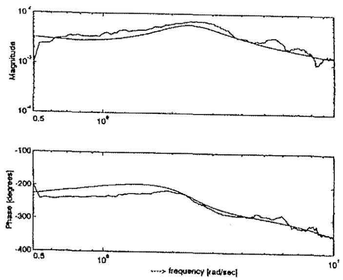
Fig 8: Comparison of BO-105 flight data and identified frequency response -  $dlat$  to  $q$
