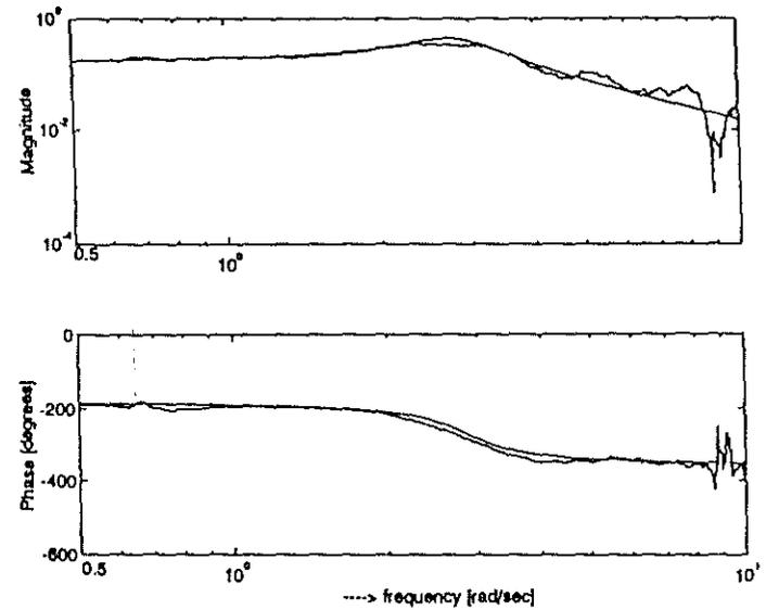
Fig 7: Comparison of BO-105 flight data and identified frequency response -
