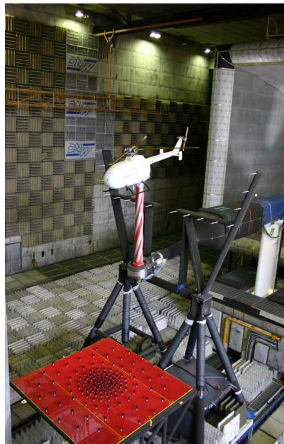
Figure 1: Bo-105 helicopter wind tunnel model, acoustic array, and microphone traverse in the DNW 8m by 6m open test section
