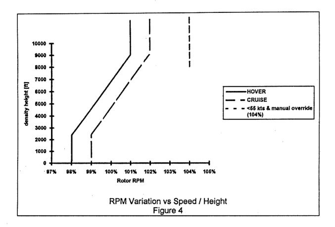
Engine 2 is controlled in such a way, that both engines will have the same torque or the pilot can choose a fixed torque split (If the switch on the collective is on 104%). With this task it is possible (in low altitudes) to operate the two engines with the same torque where the max. torque is limiting the max. power. In high altitudes, where the N1 is limiting max. power, it is possible to fly with different torque but with equal delta N1 which is then the limiting parameter.
