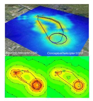
*Figure 16 - Mission profiles simulation performed with coupled PHOENIX-IESTA platforms – noise footprint*
