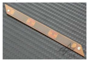
Fig. 4 - Piezoelectric actuators for blade twist
