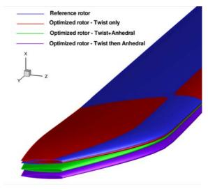
Fig. 6 - Passive Rotor Optimisation (example)
