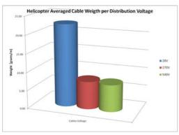
*Fig.* 8 - *Cable weight reduction with 270 & 540 VDC network standards*
