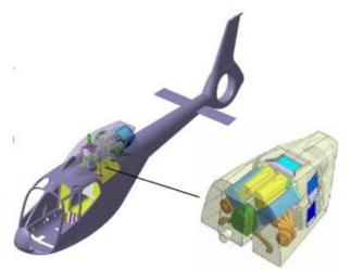
Fig.11- Preliminary demonstrator engine EC120 installation layout
