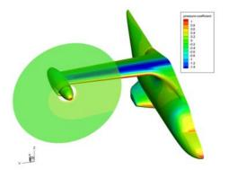
Fig. 8 - ERICA cruise flight CFD computation (CODE-Tilt)
