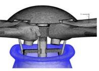
Fig. 7 - Unstructured grid for EC135 main rotor hub
