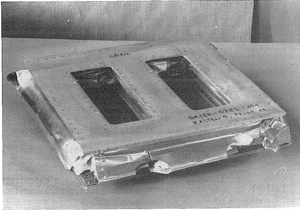
Figure 3-3. Box Type Sandwich Specimen after Dynamic Test
