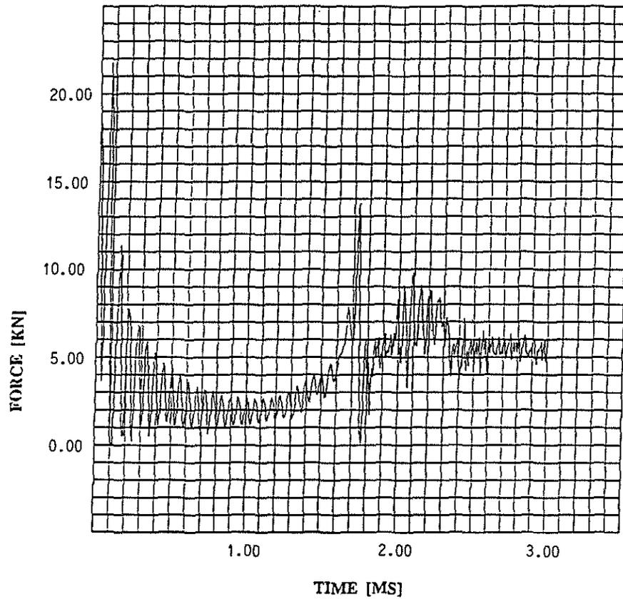
Figure 5-3. Load Time History of Numerical Simulation
