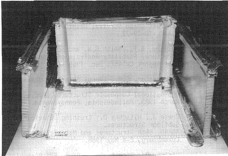
Figure 6-5. All-Sandwich Specimen after Drop Test
