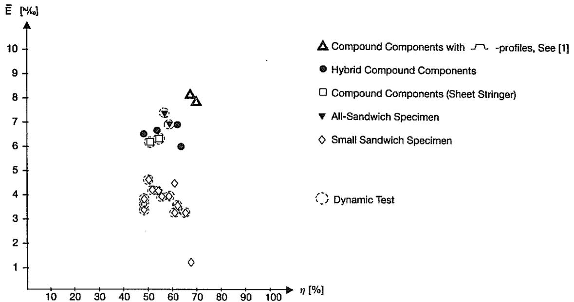
Figure 6-1. Specific Energy Absorption and Efficiency of Various Specimens
