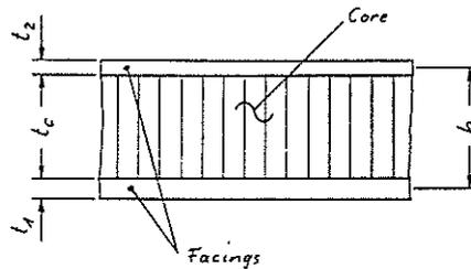
Figure 4-2. Dimensions of Sandwich
