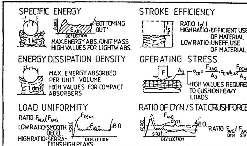
Figure 2-2. Key Parameters of Energy Absorption
