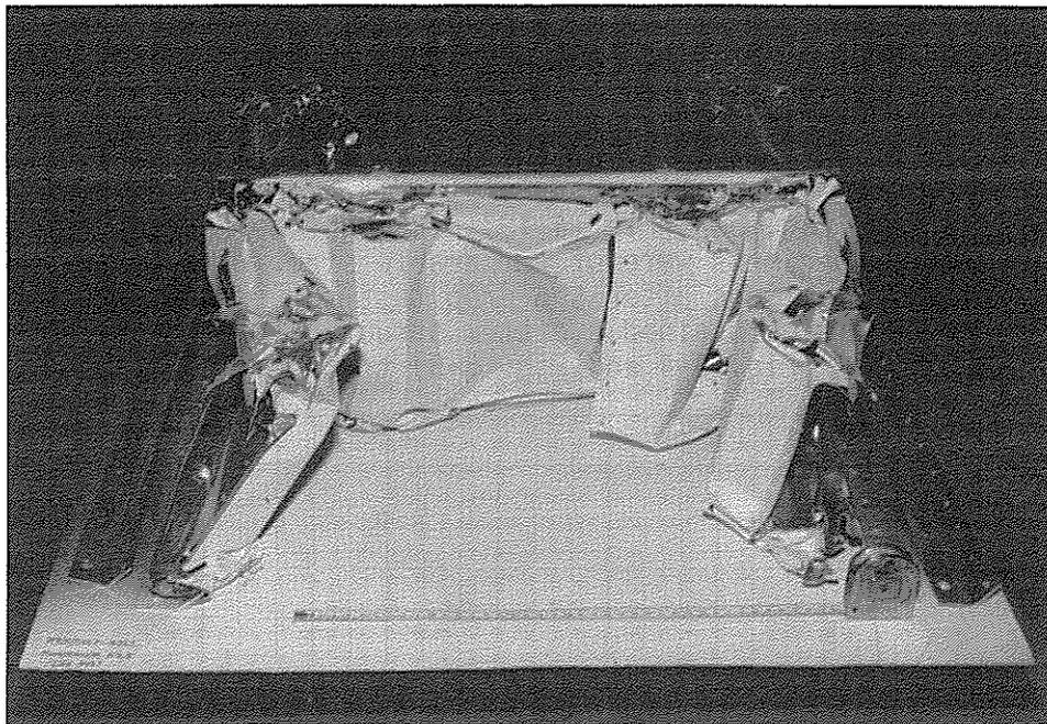
Figure 6-4. Sheet Stringer Specimen after Drop Test
