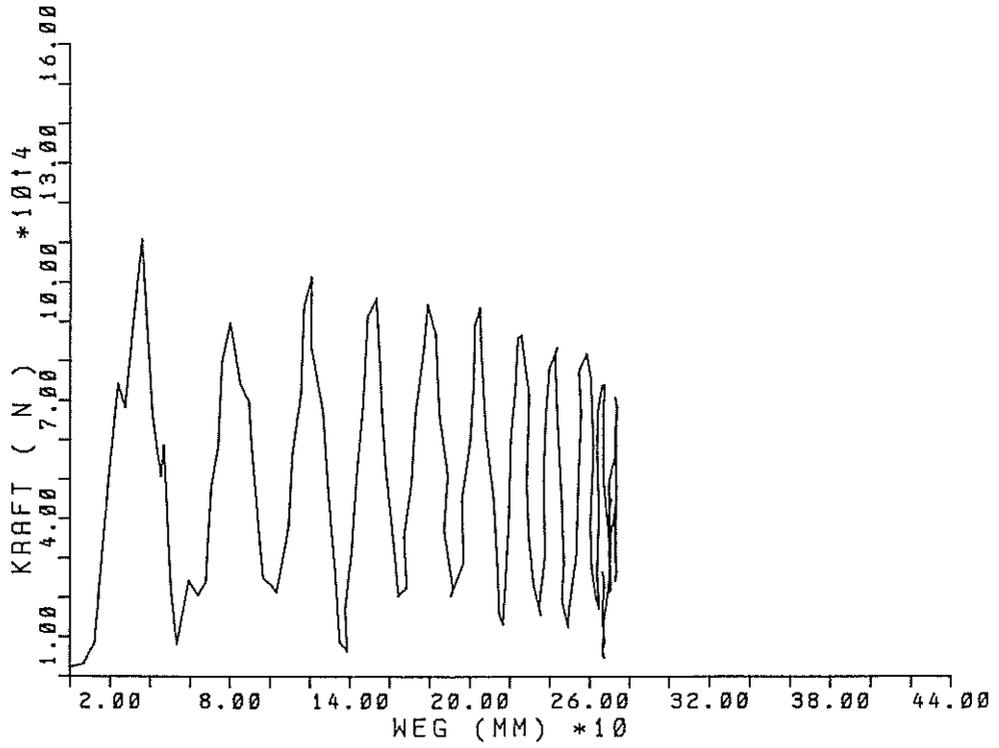
Figure 6-3. Dynamic Load-Stroke Curve of Sheet-Stringer Specimen
