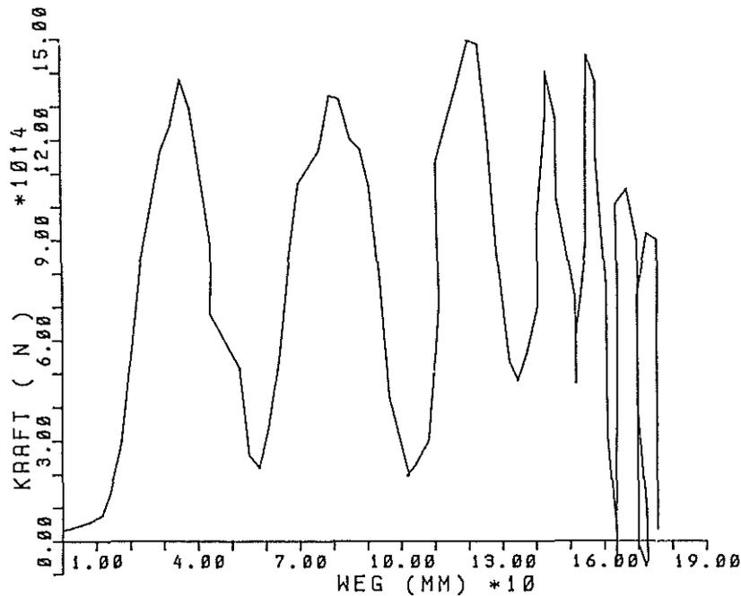
Figure 4-12. Dynamic Load-Stroke Curve of All-Sandwich Specimen
