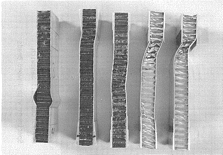
Figure 4-3. Small Sandwich Specimens
