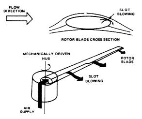
Figure 4 - Circulation Control Rotor-Basic Concept
