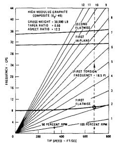
Figure 17 – X-Wing Rotor Blade Frequency Characteristics
