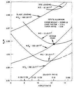
Figure 12a - Blade Weight/Gross Weight Ratio
