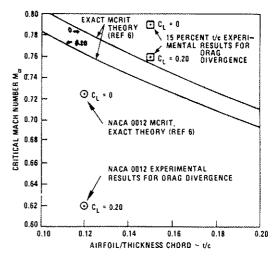
Figure 2 – Compressibility Characteristics of Two Dimensional C.C. Airfoils at Zero Angle of Attack
