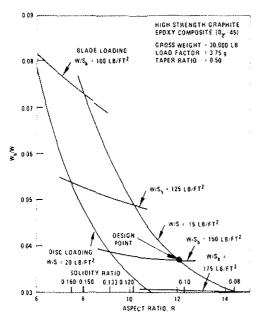
Figure 13a - Blade Weight/Gross Weight Ratio
