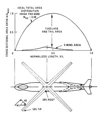
Figure 3 - X-Wing Transonic Design Features (Approximate Drag Divergence Mach = 0.89)
