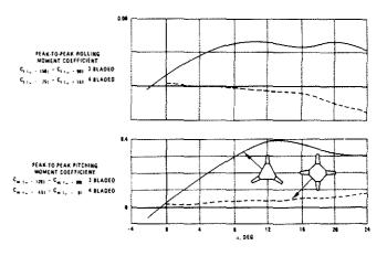
Figure 18 – Effect of Four Blades on the Reduction of Peak-to-Peak Moments during the Rotor Revolution (Reference 5)
