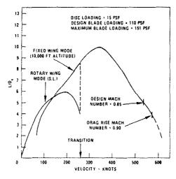
Figure 9 – X-Wing Aircraft Equivalent Lift-to-Drag Ratio
