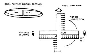
Figure 5 – Dual Blowing Concept for Transition Through High Advance Ratios
