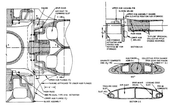
Figure 14 - X-Wing Dual Cross-Spar Rotor Hub Structural Design
