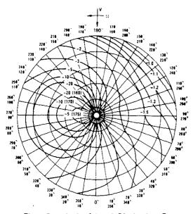
Figure 7a - Angle of Attack Distribution, Degrees
