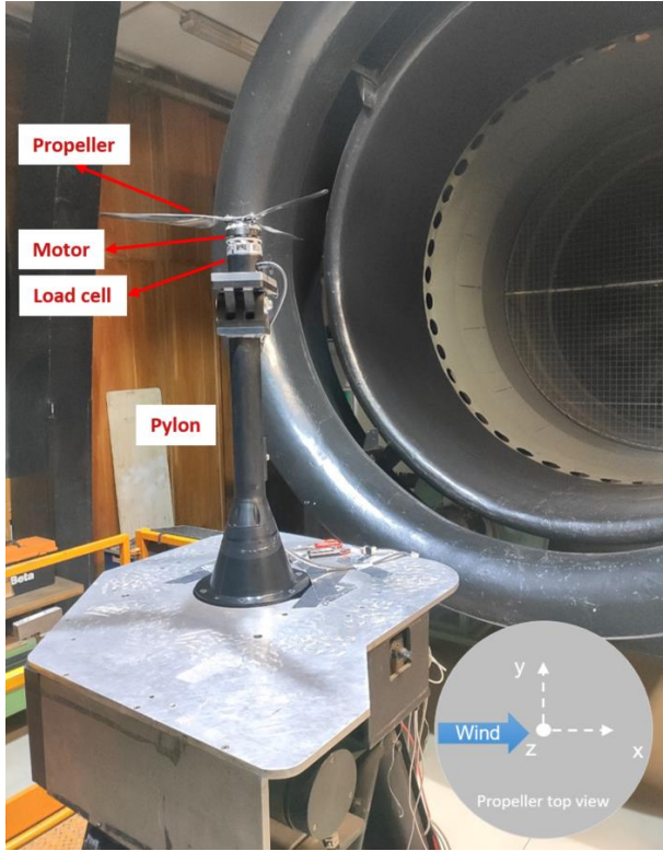
Figure 1: Wind tunnel test rig consisting of a supporting pylon structure and an LTU; system of reference (bottom right).
