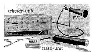
Fig. 16 Flow Visualization Gun apparatus
