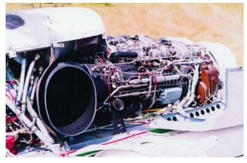
The emergency power of VK-2500 engine enables to continue the interrupted take-off. The new engine's service life is also extended. The enhanced performance of VK-2500 engine gives hovering ceiling gain (especially under high temperature conditions) and improves the helicopter performance.
