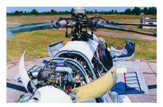
The second stage envisages the upgrade of the rotor system. The helicopter will be equipped with new blades made of composite materials. Nowadays Mil Moscow Helicopter Plant has completed the blades' flight tests which proved their aerodynamic characteristics.
