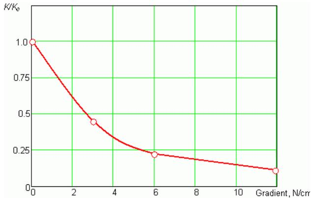
Figure 8: Transfer function parameter adjustment for the effect of inceptor force gradient.
