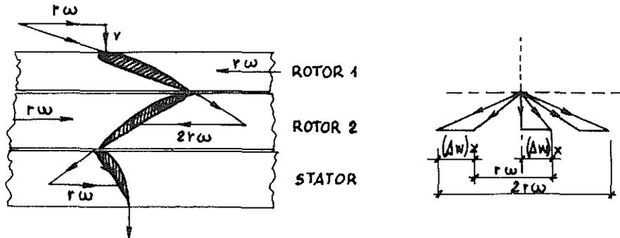
Fig. 3 - Flow velocity diagram in the proposed counterrotating rotor system.
