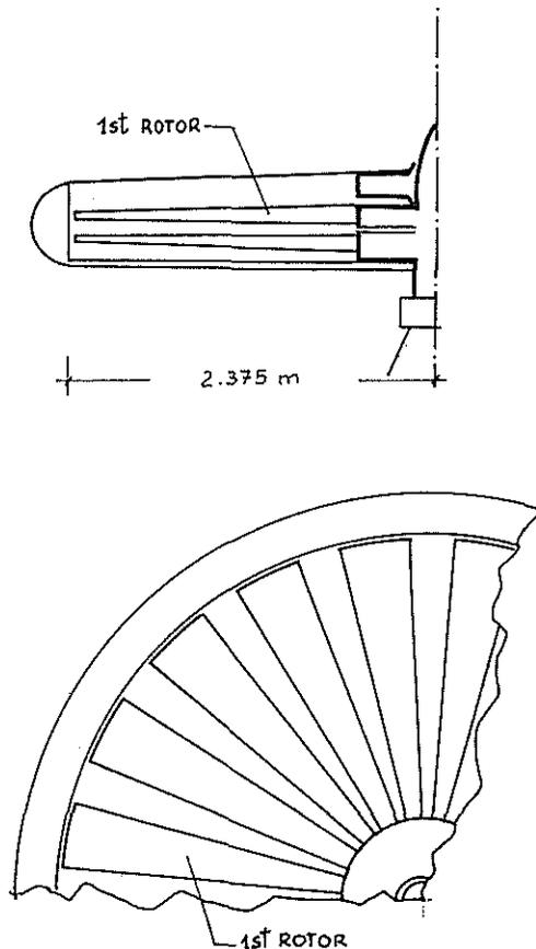
Fig. 2 - Ducted composite counterrotating rotor system.
