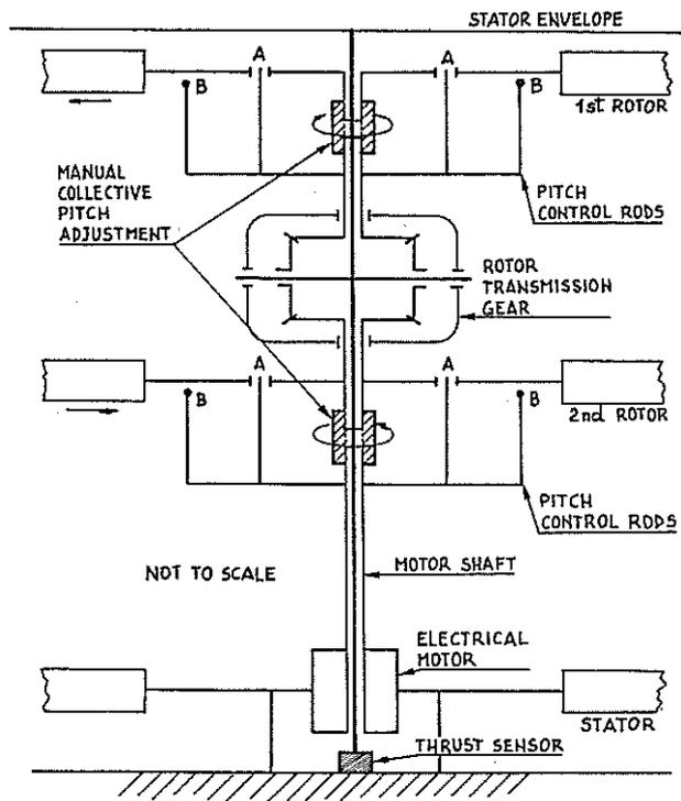
Fig. 4 - Sketch of the rotor power transmission for the scale model.
