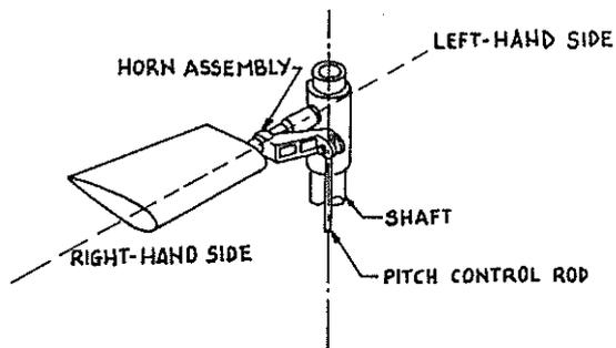
Fig. 5 - Blade collective pitch control linkage.
