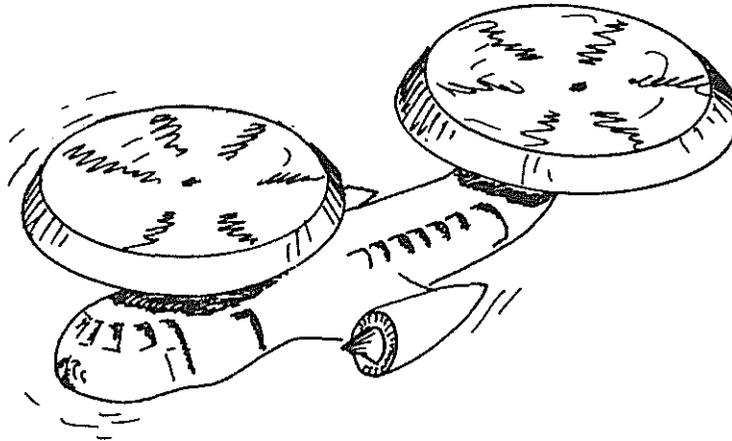
Fig. 1 - Solution for High Altitude Ducted Counterrotating High Solidity Rotors.
