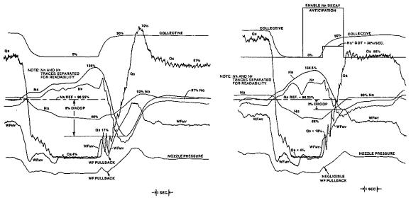
WAVEOFF FROM AUTOROTATION WITH THE BASELINE FADEC CONTROL WAVEOFF FROM AUTOROTATION WITH ROTOR DECAY ANTICIPATION
