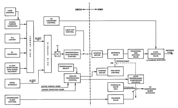
Figure 5 FADEC SIMPLIFIED FUNCTIONAL BLOCK DIGRAM
