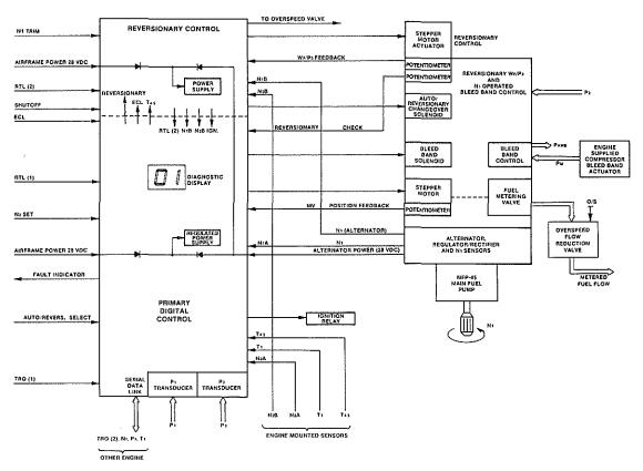
Figure 4 FADEC INTERFACE BLOCK DIAGRAM
