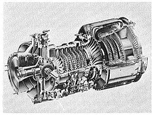
Figure 2 LYCOMING T55-L-712 TURBOSHAFT ENGINE
