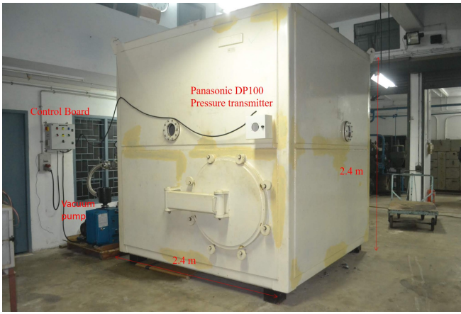
Figure 1: 2.4m×2.4m×2.4m Vacuum chamber
