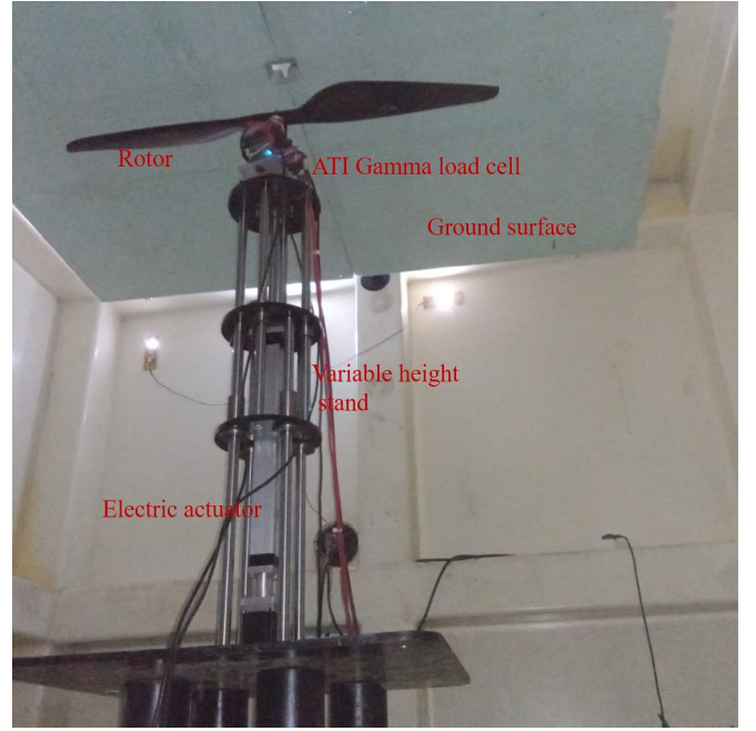
Figure 5: Ground effect setup: Inverted flow configuration
