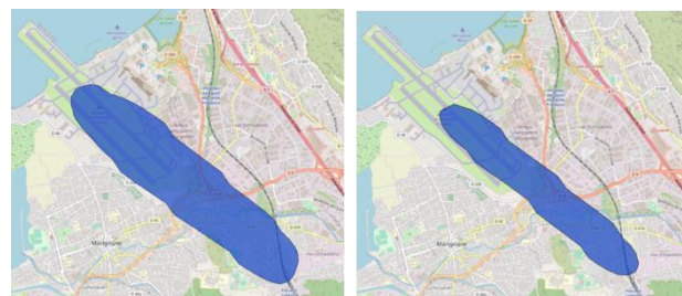
Figure 24: 80dB SEL contour in approach for reference H/C (left) and new H/C design (right).
