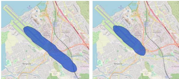
Figure 25: 80dB SEL contour in approach for an H/C with a modified rotational speed on reference procedure (left) and a LNP (right).
