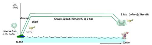
Figure 16: Standard Mission Profile of SUAV (Emergency Catch Up)
