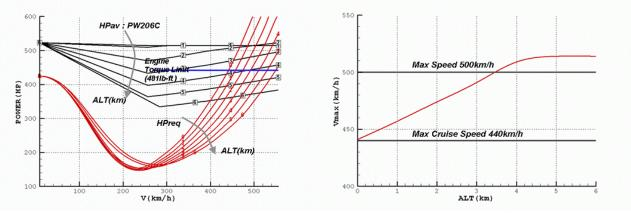
Figure 6: Speed vs. Required Power
