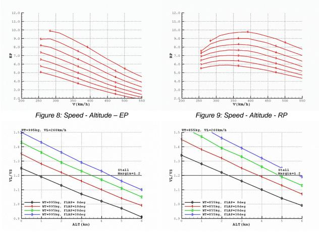
Figure 10: Altitude vs. Stall Margin (Weight =995kg) Figure 11: Altitude vs. Stall Margin (Weight=855kg)
