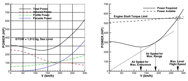
Figure 13: Speed vs. Required Power
