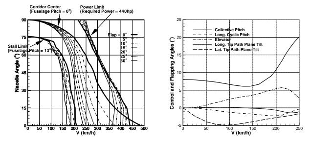
Figure 14: SUAV Conversion Corridor Variation with Figure 15: Control and Flapping Angle Variation along Flap Deflection Corridor Center (Flap=25°)
