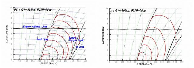
Figure 12: Flight Envelope (Weight=995kg, Flap =0°, Specific Excess Power (PS) & Load Factor (n))
