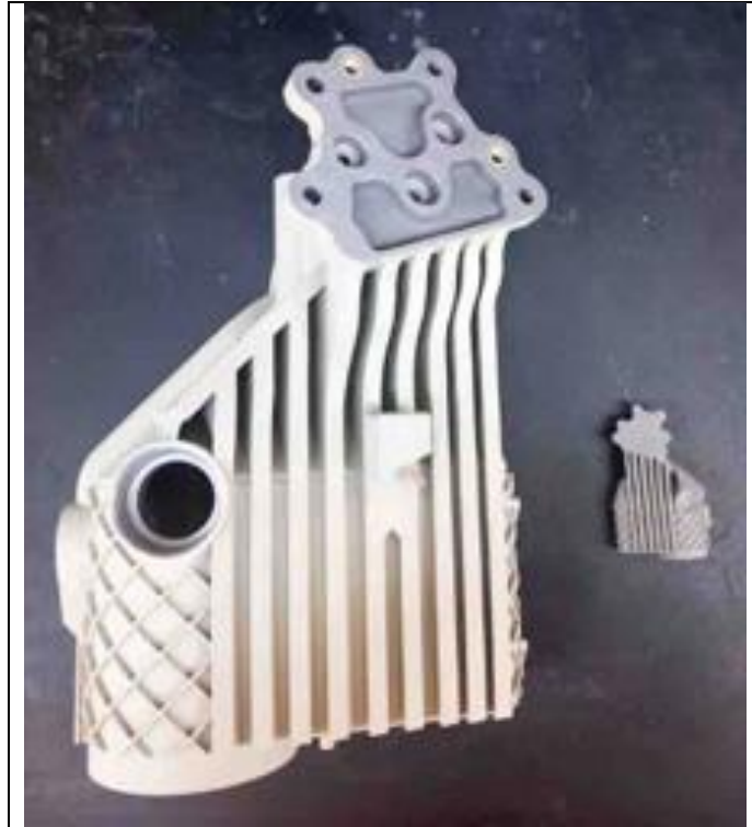
Figure 12. 3D printed Auxiliary tank in LPBF (left) and its 1:5 scaled model in BJ (right)
