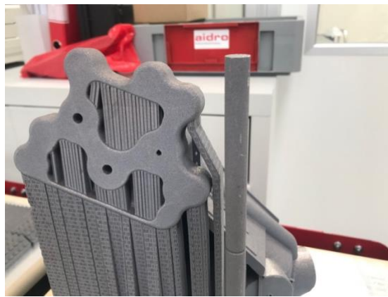
Figure 5. Support structures and test coupon 3D printed with the component
