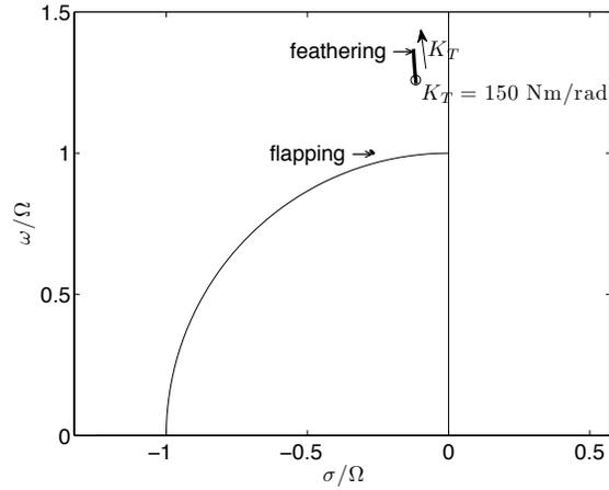
Figure 9: Root locus as a function of  $K_T$ ;  $\mu = 0$ ,  $K = 3,610$  Nm/rad.
