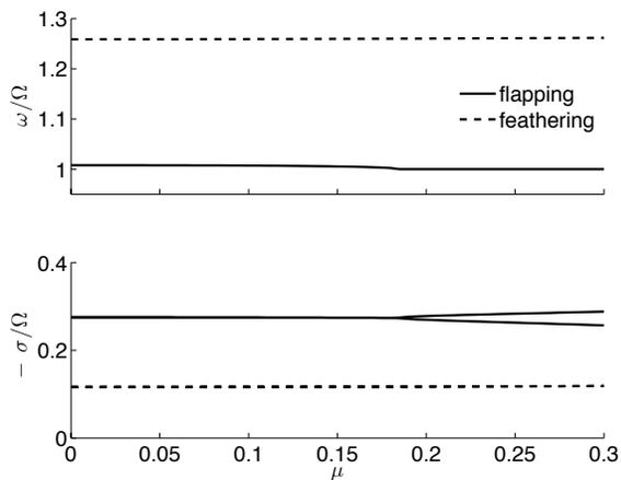
Figure 12: Frequency and damping as a function of  $\mu$  from Floquet analysis for  $K = 3, 610 \text{ Nm/rad}$ .
