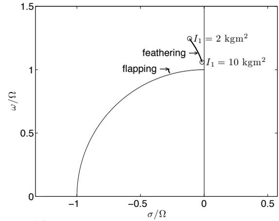
Figure 10: Root locus as a function of  $I_1$ ;  $\mu = 0$ ,  $K = 3,610$  Nm/rad.
