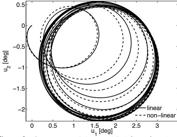
Figure 2: Comparison of the simplified (linear) and general (nonlinear) rotor model responses to a longitudinal cyclic command  $\theta_{SW} = 5$  deg;  $\mu = 0$ ,  $K = 3,610$  Nm/rad.
