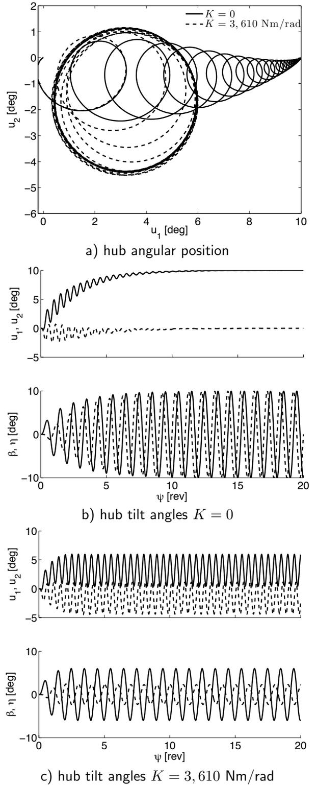
Figure 4: Response to a longitudinal cyclic command  $\theta_{SW} = 10 \text{ deg}$ .
