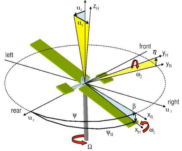
Figure 1: Rotor coordinate system.
