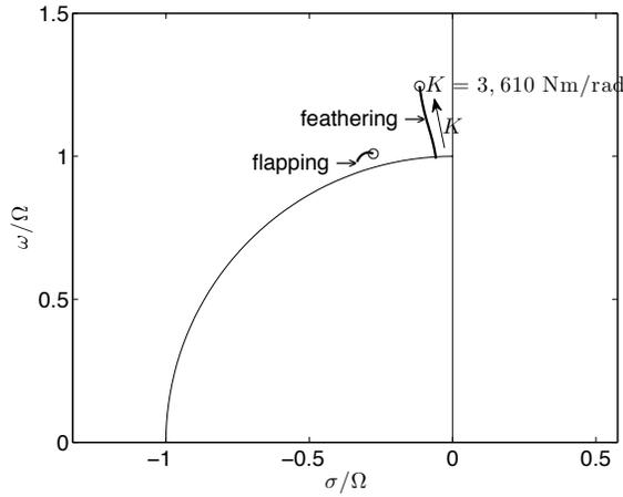
Figure 8: Root locus as a function of  $K$ ;  $\mu = 0$ ,  $k_T = 0$ .
