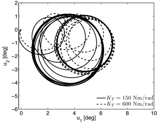
Figure 7: Response to a longitudinal cyclic command  $\theta_{SW} = 10$  deg;  $K_T \neq 0$ .
