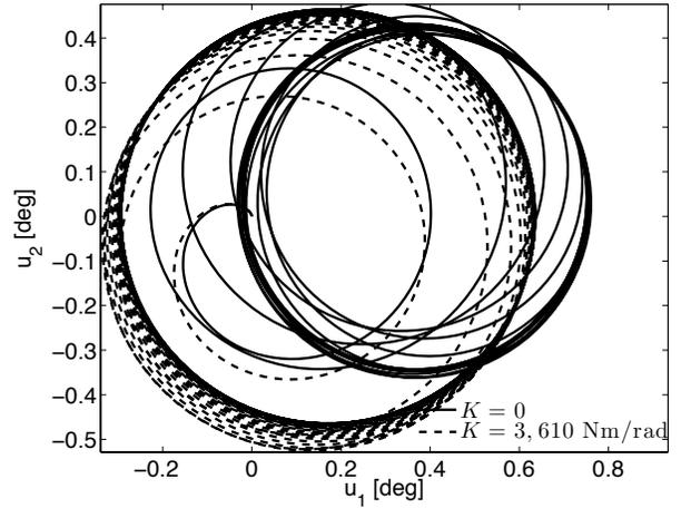
Figure 6: Response to a perturbation of the advance ratio  $\mu = 0.05$ .
