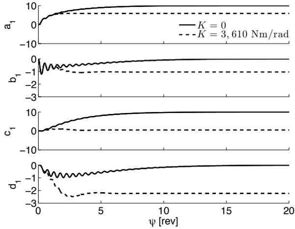
Figure 5: Response to a longitudinal cyclic command  $\theta_{SW} = 10$  deg in terms of flapping coefficients.
