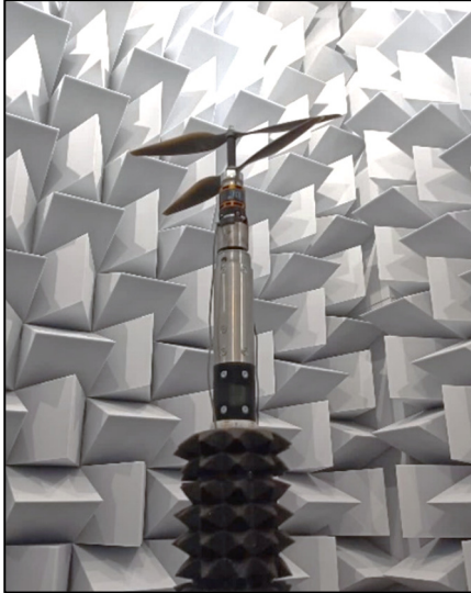
Figure 1: Test rig configuration for testing stacked rotors
