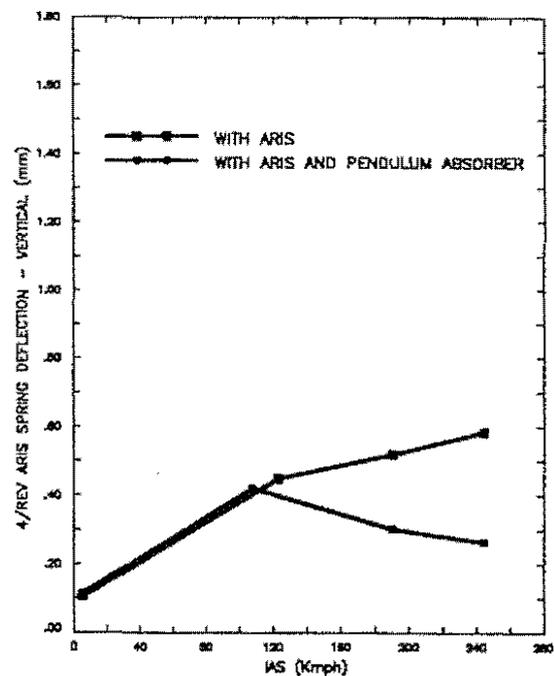
Fig. 19 : Spring Displacement With Forward Speed
