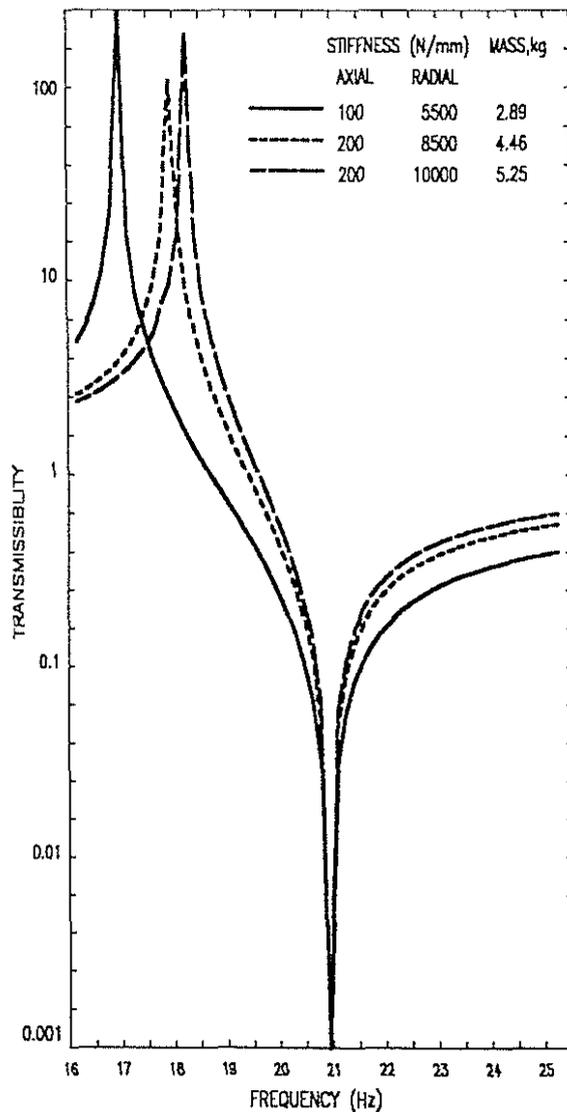
Fig 4: Transmissibility For Different Spring Stiffness
