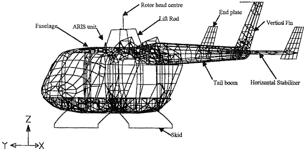
Fig. 8 : FE Idealisation of Airframe With ARIS Units
