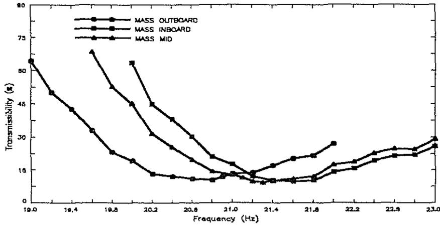
Fig. 14 Transmissibility with different Tuning Mass position
