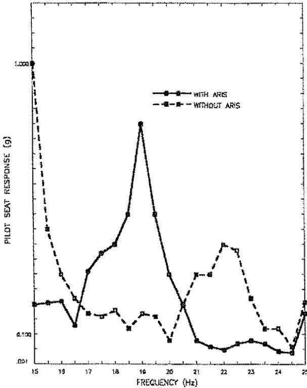
Fig. 9 : Pilot Seat Response with and without ARIS
