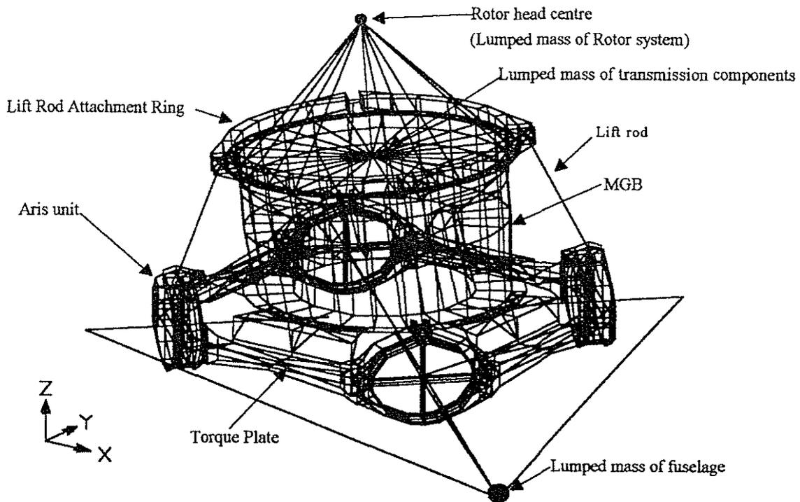
Fig.6 : FE IDEALISATION OF MGB ASSEMBLY WITH ARIS UNITS
