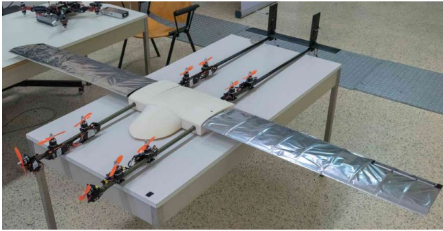
Figure 2. Lift+Cruise eVTOL drone aircraft in the lab (Ref. 17).
