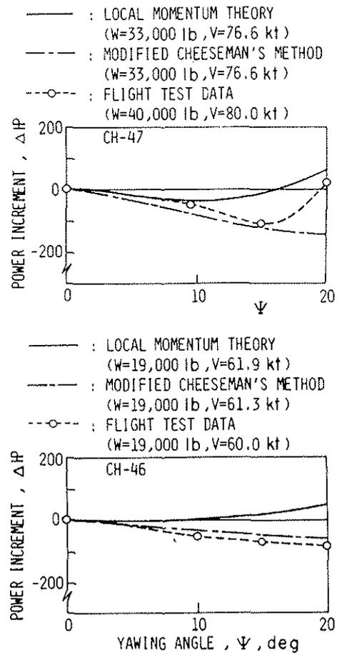
Figure 11. Comparison of theoretical results and flight test data in the power increment due to right yaw.
