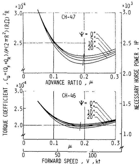
Figure 10. Necessary horse power in yawed flight. (C.G. position at center)
