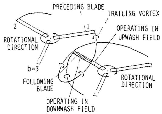
Figure 2. Interference between blades and tip vortices.
