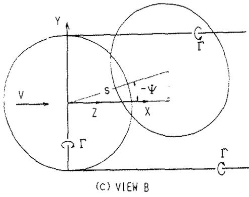
Figure 1. Vortex system of front rotor.
