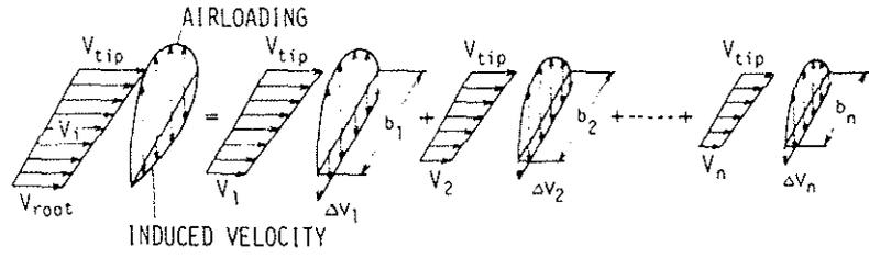
Figure 3. Decomposition of a rotary wing.
