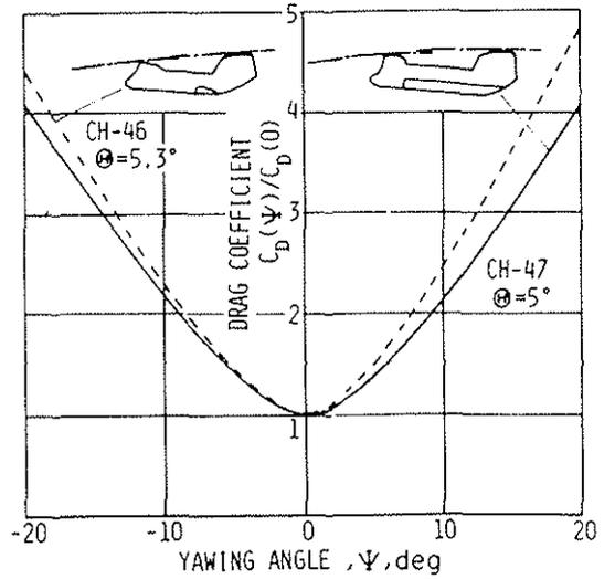
Figure 9. Parasite drag coefficients fuselage for CH-46 and CH-47 obtained from experimental data.
