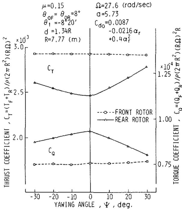
Figure 8. Performance of a tandem rotor in yaw. (No cyclic pitch inputs)
