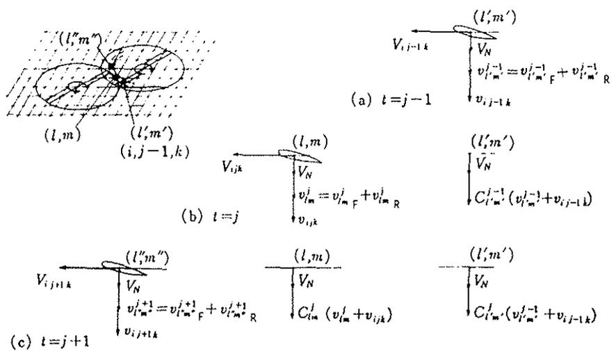
Figure 4. Successive change of the induced velocity in the rotational plane of a rotor.
